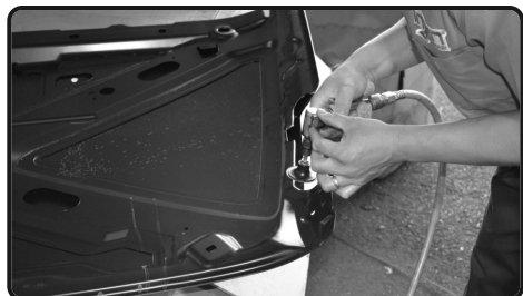
9. Use a flat grinder to straighten the edges and clean up all the metal burrs. Slowly grind back on the open. Only grind what you need for additional clearance. Please use caution and have proper safety equipment like goggles and air respirator!!!
