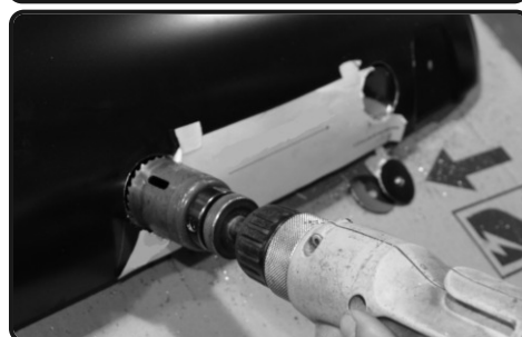
6. Using the crosshairs on the cutting template as a guide, use a 1 3/4" hole saw and drill out the two holes on the template. Make sure you drill past the second layer of the hood. Please use caution!!!
