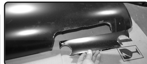
4. Locate the hood latch indentation outer tangent point and measure 0.875" left of tangent to locate supplied cutting template.
