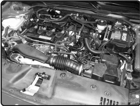
1. Stock intake system shown. Disconnect the battery before installation.
