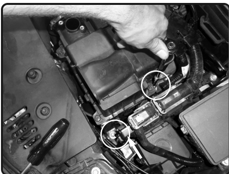
5. Loosen the 2 bolt holding in the airbox using 10mm socket and extension.
