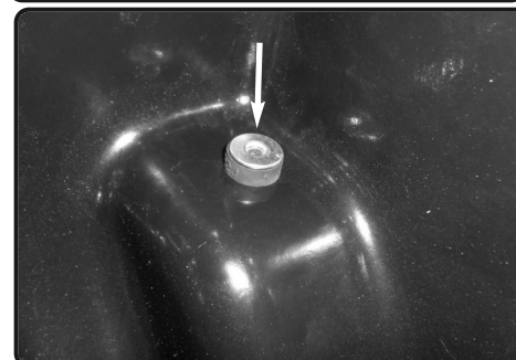
10. Now install the crush washer inside air box to the grommet.
