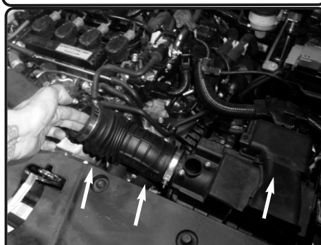
6. Pull back the intake tube from turbo housing.
