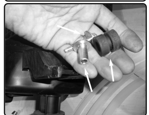
8. Remove the OEM grommet and crush washer with bolt this will be used on new injen air box.
