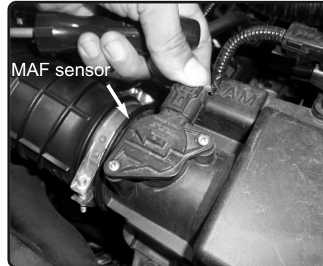
3. Disconnect the MAF sensor.
