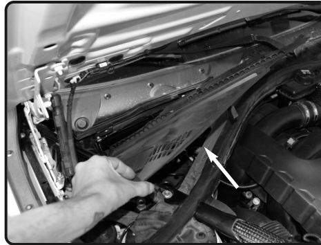
3. Loosen the engine tray and pull back weather trim seal.
