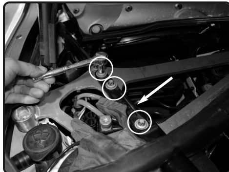
6. Loosen the 3 bolts on the end of the strut bar and remove. Continue on other side.
