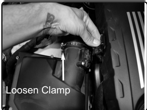
9. On passenger side, disconnect MAF sensor harness. Loosen the clamp on the air box using 7mm nut driver.
