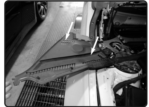
4. Lift up and turn the engine tray out of the way. This will allow for removal of the factory strut bar. Now repeat and do on other side of vehicle.
