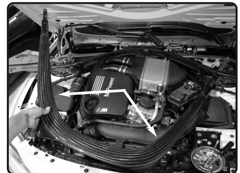
8. Now lift up and remove the factory strut bar. This will now have access for the intake systems.
