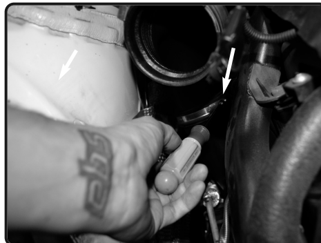
11. Loosen the clamp on the turbo housing using 7mm nut driver. Now lift up and remove passenger side intake tube from vehicle.
