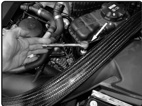
5. Loosen the 10mm bolt holding the strut bar on coolant reservoir.
