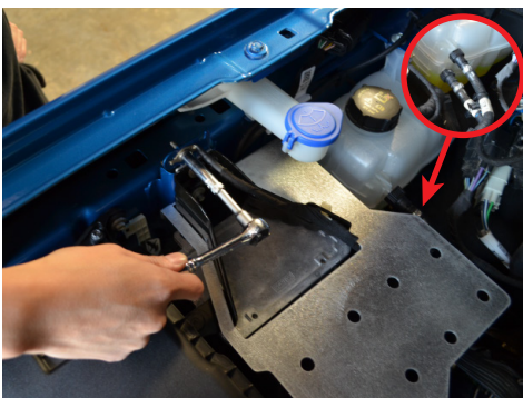
10. Resecure the ground wire with the OEM bolt. Ensure the bracket does not hit any coolant lines.
