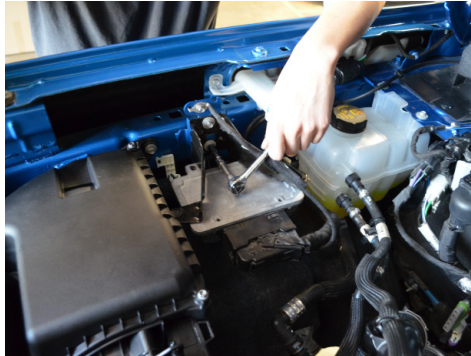
5. Remove the 2 bolts securing the OEM ECU bracket and the bolt securing the ground wire.
