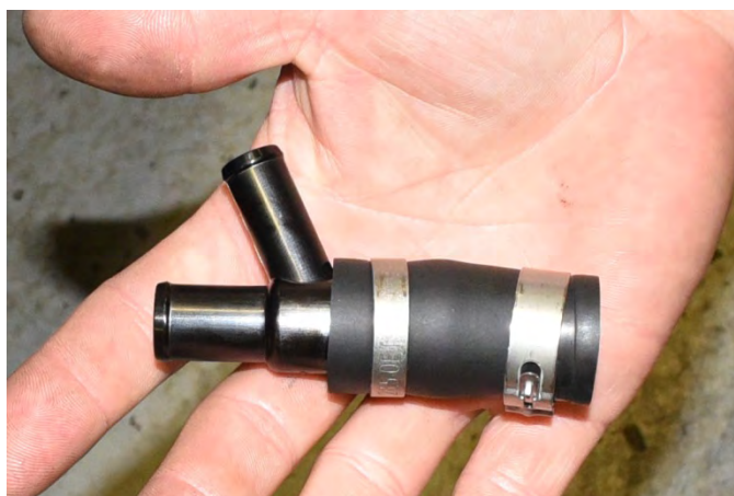
Drain fitting installed into the OEM \frac{3}{4} " hose
