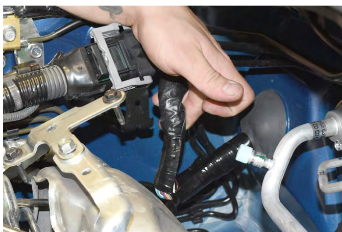
Main wiring harness shown after cutting tape
