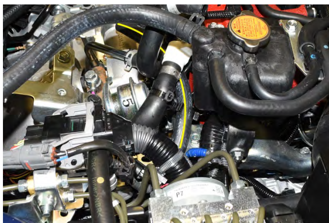
Yellow stripe shows routing to turbo coolant line
