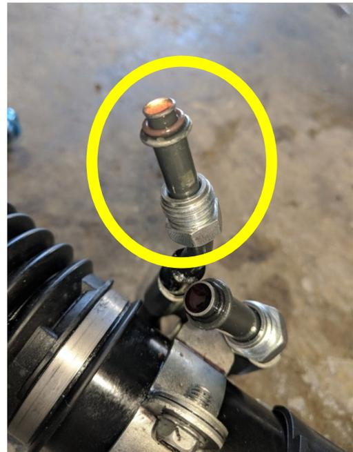
2. Attach the straight-fitting side of the stainless-steel line to the male side of the male-to-female fitting. Tighten this connection to 16.25 ft-lb.
