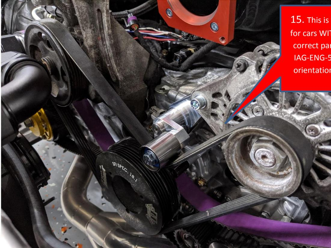
15. This is the correct belt routing for cars WITH power steering. The correct part number for this kit is IAG-ENG-5211. Note the correct orientation of the tensioner arm.
