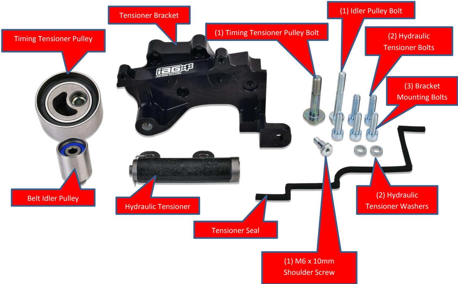
1. Apply included foam seal to the back side of the large tensioner bracket. This seal goes between the block and the tensioner bracket.
