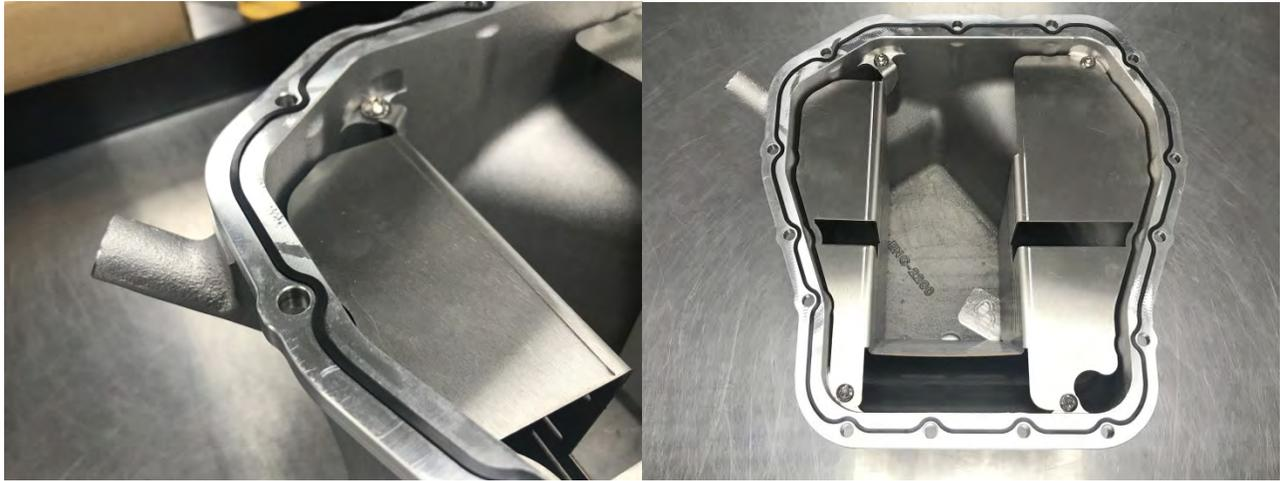
Figure 4 - O-ring Seal
