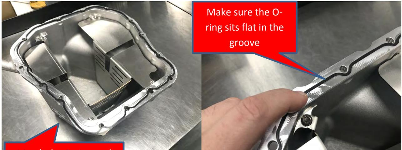
Figure 3 – O-ring Seal
