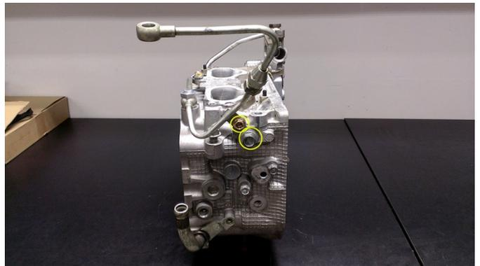
2. Install the supplied oil plug in the **top** oil port. Use a 12mm crush washer between the head and plug. Torque the plug to 24 <sup>ft</sup>/<sub>lbs</sub>.
