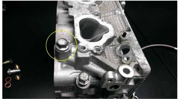
7. Assemble one 12mm banjo on the bottom port of the tee fitting. The braided line with the straight fittings is installed on the middle port and the braided line with the 90° fitting is installed on the top port as shown. The 90° fitting will be installed on the top of the turbo. It is important that the face of the banjo fitting be parallel with the side of the t-fitting. Tighten all 3 fittings with a  $\frac{9}{16}$ " wrench.
