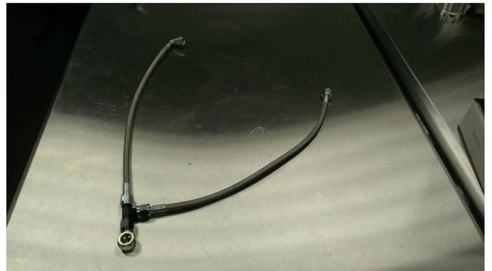
8. Using the banjo bolt that came out of the back of the head, assemble the tee fitting on the back oil port of the head as shown. Use a thinner washer between the head of the banjo bolt and the banjo. Then use the thicker washer between the banjo and the engine. This is the only place to use a thick washer.
