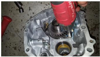
10. Install the output shaft into the housing being sure to lubricate the bearings with gear oil. Then install it onto transmission with 4 bolts (2 top and 2 bottom) and torque bolts to 48nm (35.4ft lbs). Make sure the shaft is not loose and spins smoothly, if it is loose or too tight it will require shimming.
