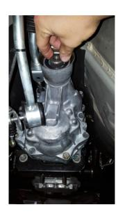
11. Remove the snap ring on the drive gear and press off the bearing. Next press the bearing onto the new drive gear and re-install the snap ring. There are shims on the drive gear, these will be re-used so do not lose them!
