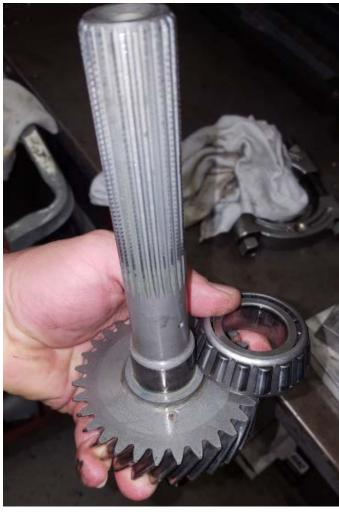
8. Press the bearings onto the new output shaft. You can use the old bearing races to support the bearings when pressing them onto shaft. Spin the bearing while pressing it onto shaft making sure the bearing doesn't bind or get damaged during install.
