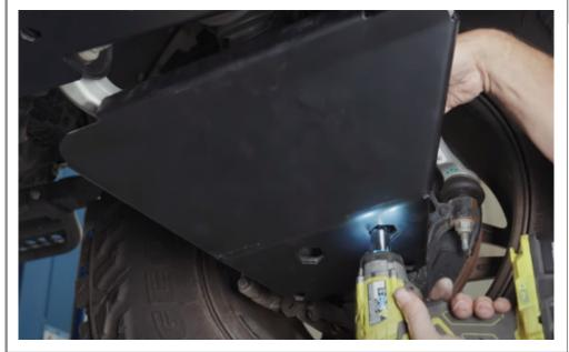
Step 3 Reinstall the strut bolts or nuts and tighten.
