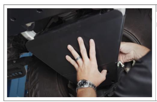
Step 2 Hold up skid plate so the holes align with strut.
