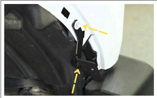
Install the bracket onto the fender.
