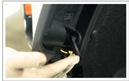
Remove the front fender flare from the drivers side.
