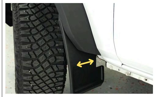
Adjust Mud Flap to align with fender flare, then tighten the mudflap hardware. (10Nm)
