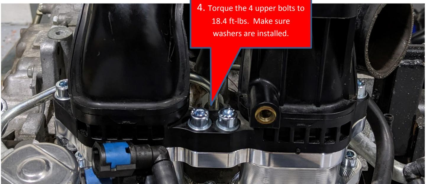
4. Torque the 4 upper bolts to 18.4 ft-lbs. Make sure washers are installed.
