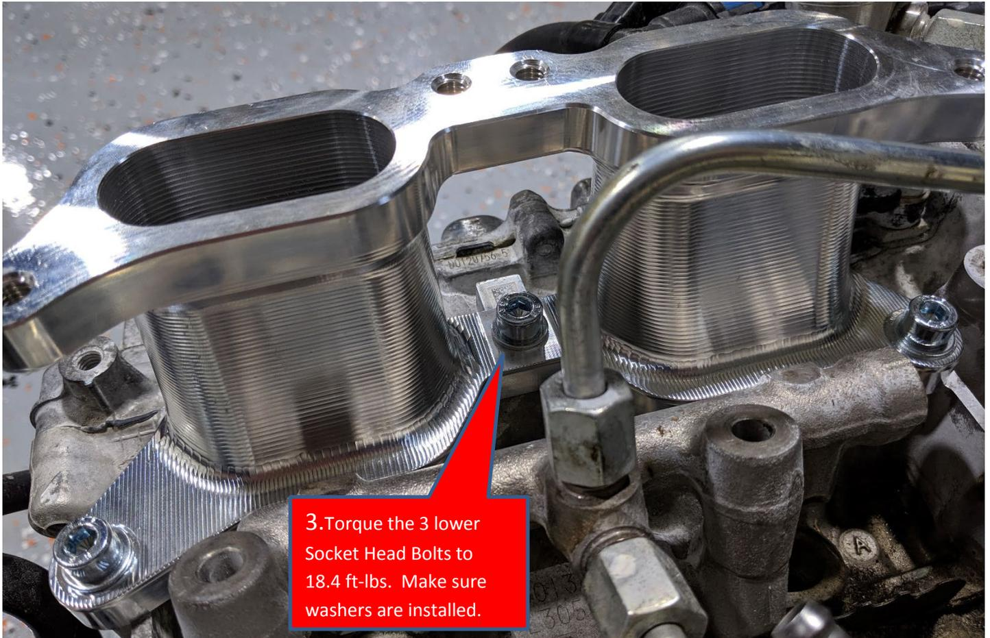
3. Torque the 3 lower Socket Head Bolts to 18.4 ft-lbs. Make sure washers are installed.
