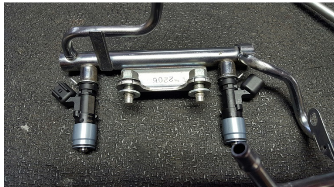
2a. Shows (x2) OEM hex head bolts, placed through the OEM fuel rail mounting points with (x2) 8mm washers added as spacers to each side.
