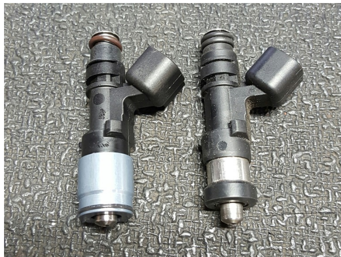
Picture above shows the New Injector Dynamics top feed injector body (left) versus the old ID injector body (right).
