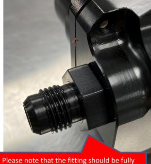
flush when installed properly. Torque these
