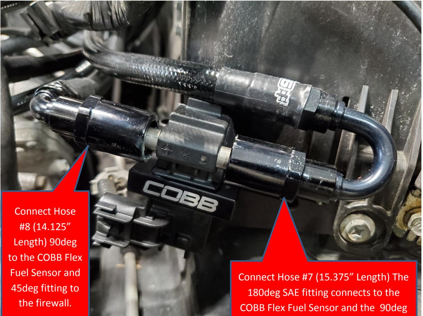
Connect Hose #8 (14.125" Length) 90deg to the COBB Flex Fuel Sensor and 45deg fitting to the firewall.
