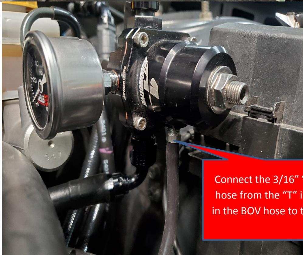
Connect the 3/16" Vacuum hose from the "T" installed in the BOV hose to this port.
