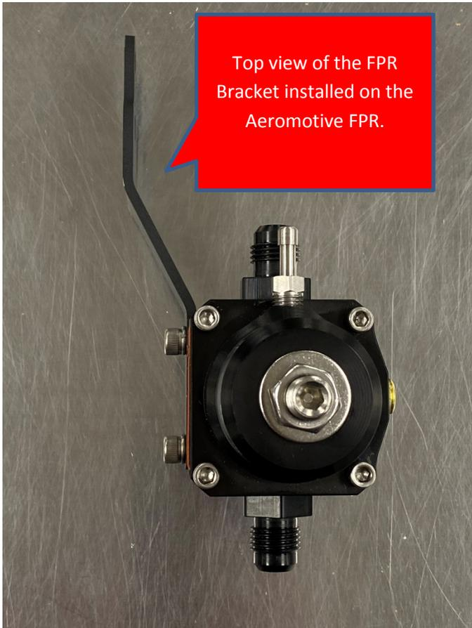
Top view of the FPR Bracket installed on the Aeromotive FPR.
