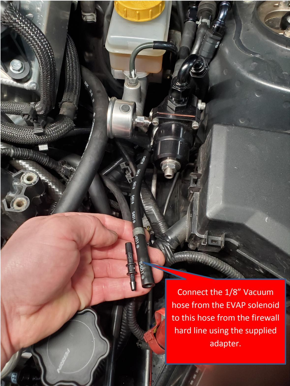
Connect the 1/8" Vacuum hose from the EVAP solenoid to this hose from the firewall hard line using the supplied adapter.
