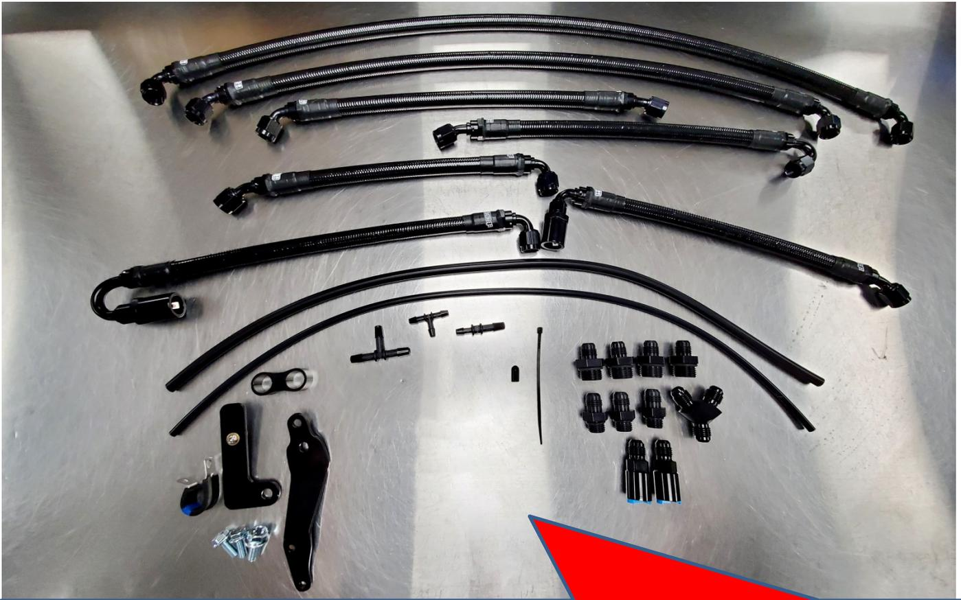
This is all the parts laid out. Please note that each hose is identified by overall length and type of fitting used. You will see on the next page how each hose is measured and how you can identify the proper hose. We will refer to each hose as "Hose 1, Hose 2, Hose 3, etc."
