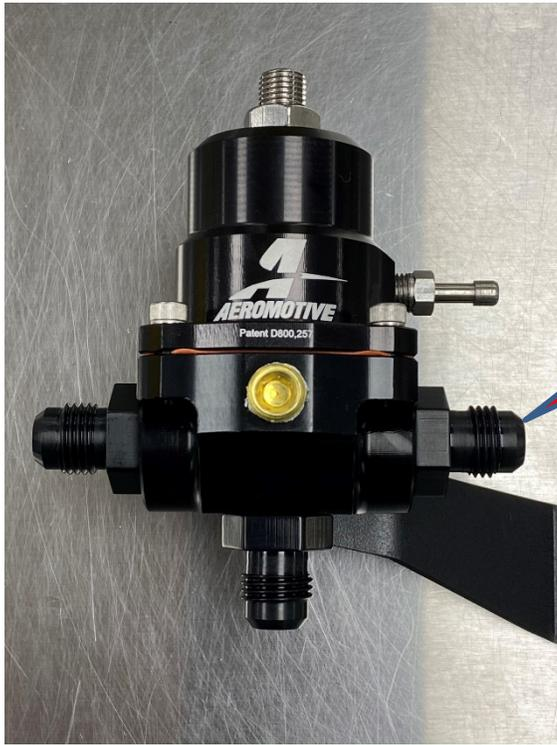
All 3 Fuel Fittings (-6 ORB to -6 AN) should be already installed, if not, install now with lube and torque to 16 ft/lbs. If used, install your Fuel Pressure Sensor or Gauge in the NPT port on the front now.
