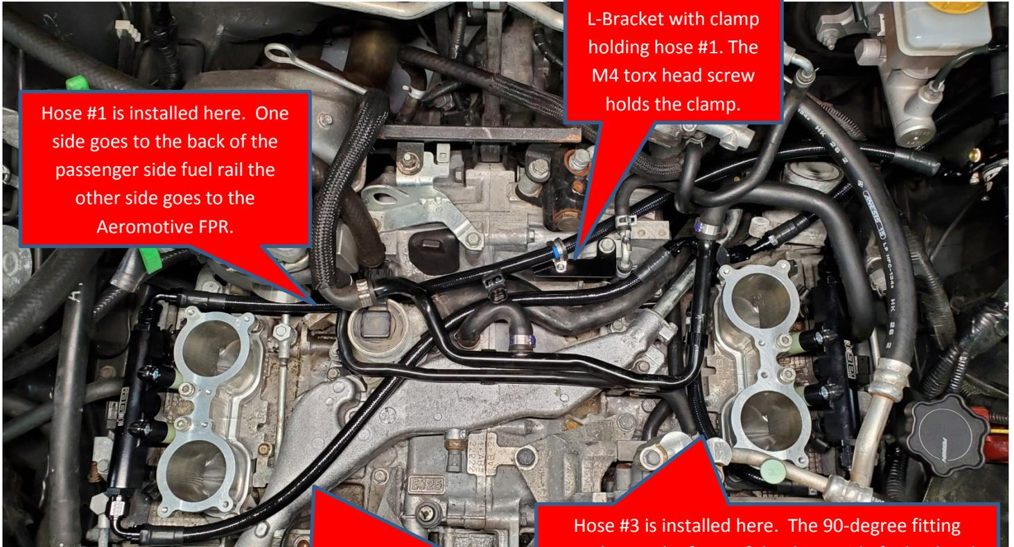
Hose #1 is installed here. One side goes to the back of the passenger side fuel rail the other side goes to the Aeromotive FPR.
