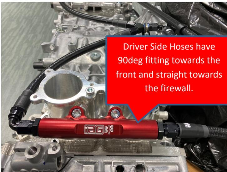
Driver Side Hoses have 90deg fitting towards the front and straight towards the firewall.
