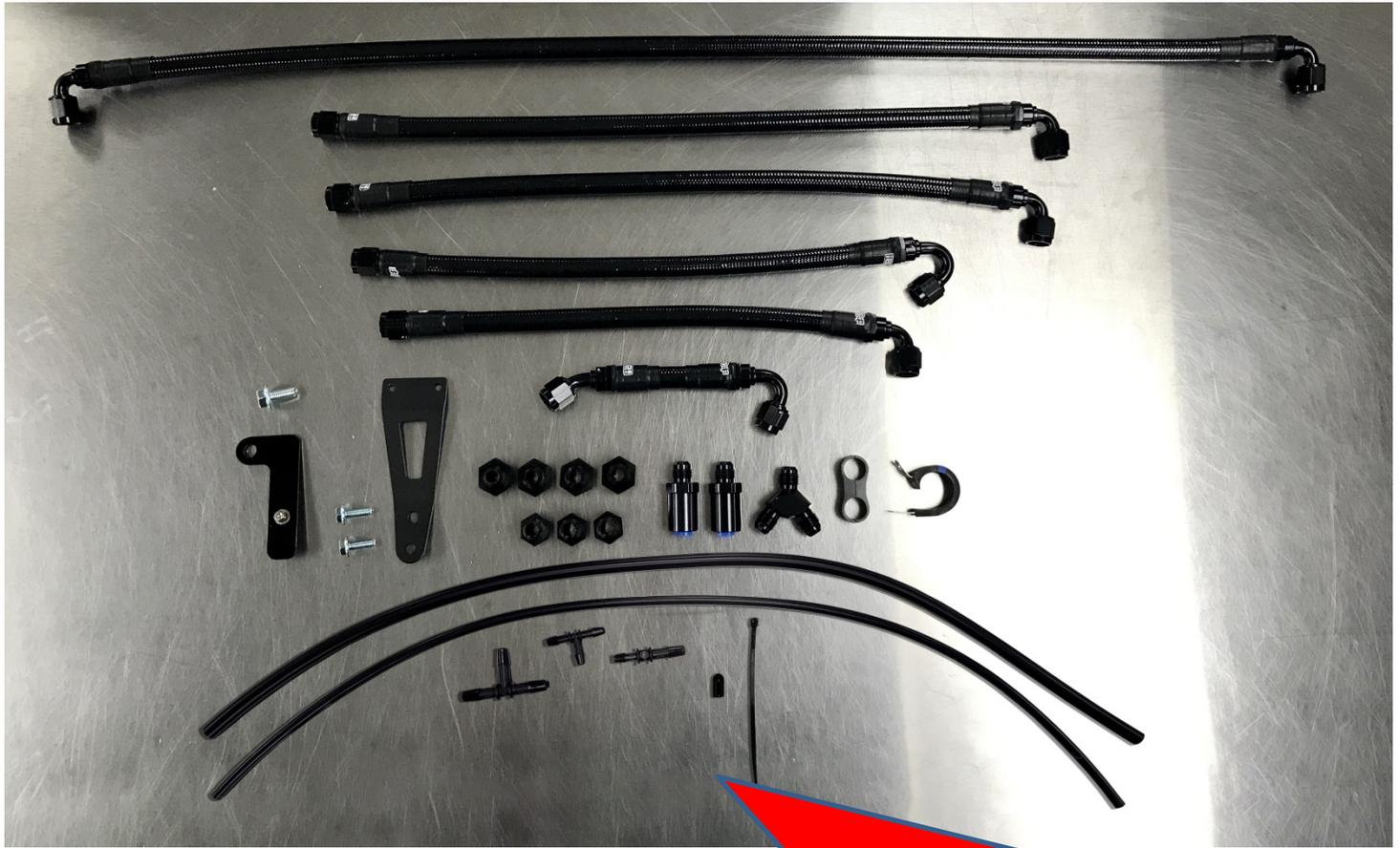
This is all of the parts laid out. Please note that each hose is identified by overall length and type of fitting used. You will see on the next page how each hose is measured, and how you can identify the proper hose. We will refer to each hose as "Hose 1, Hose 2, Hose 3, etc."
