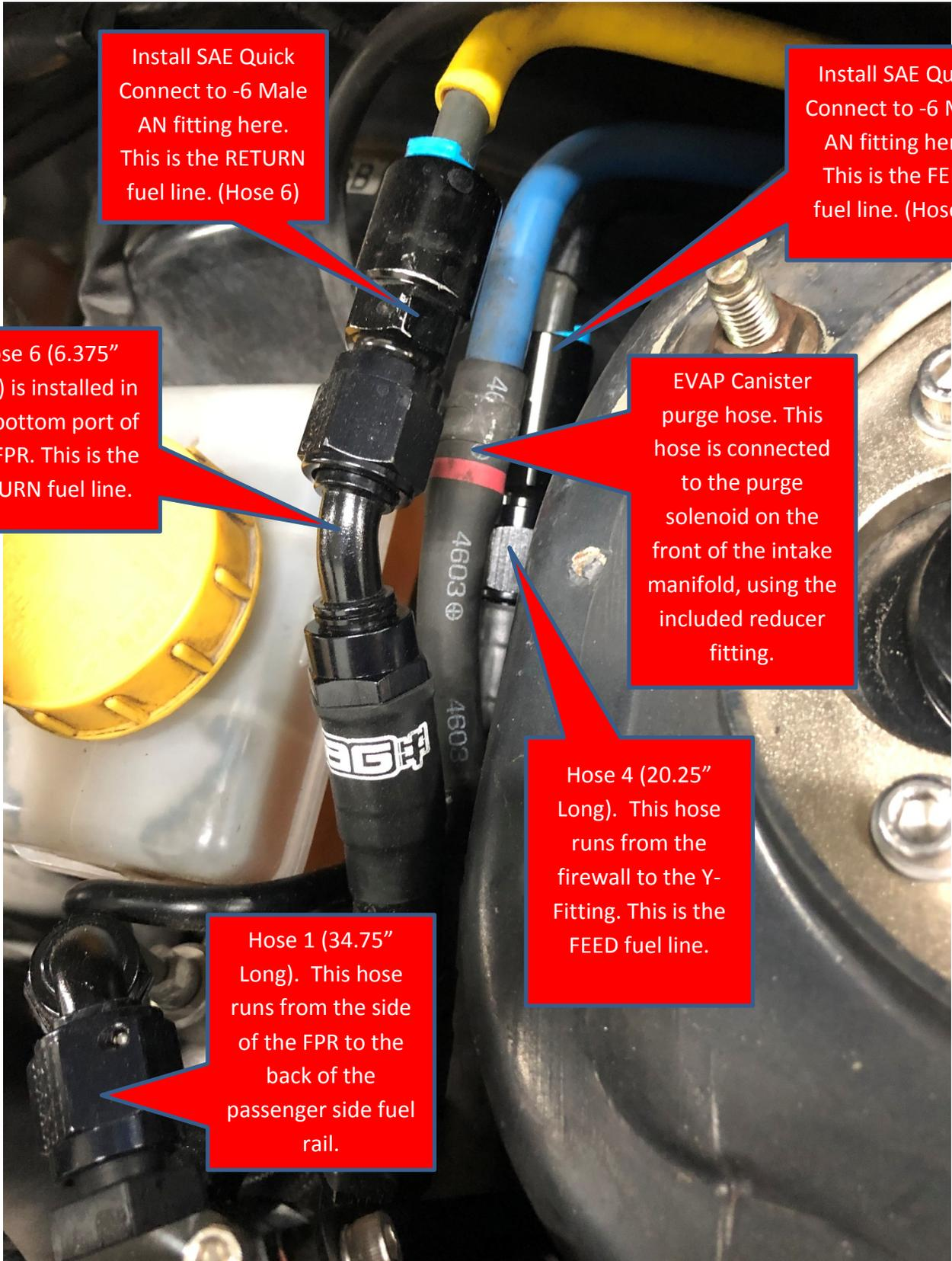
Install SAE Quick Connect to -6 Male AN fitting here. This is the RETURN fuel line. (Hose 6)
