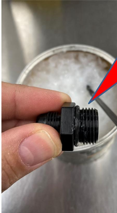
ALWAYS apply lube to all O-rings for this installation. Dry O-rings can tear and that's bad.
