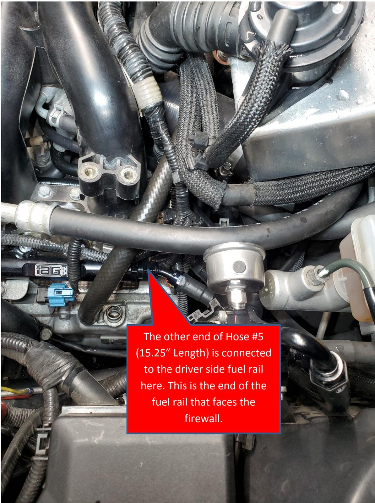
The other end of Hose #5 (15.25" Length) is connected to the driver side fuel rail here. This is the end of the fuel rail that faces the firewall.
