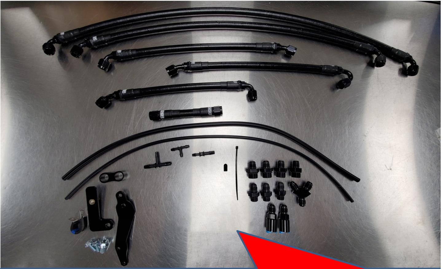
This is all the parts laid out. Please note that each hose is identified by overall length and type of fitting used. You will see on the next page how each hose is measured and how you can identify the proper hose. We will refer to each hose as "Hose 1, Hose 2, Hose 3, etc."
