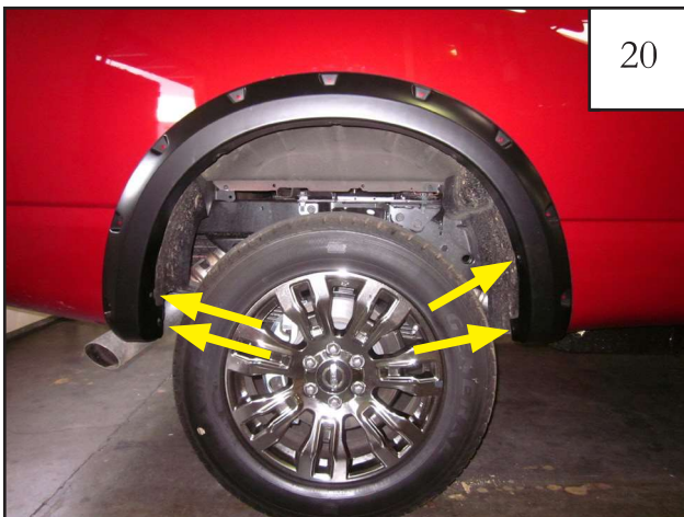
20 Install 4 supplied screws (SW1-0049) through holes in flare and into the existing factory holes.
