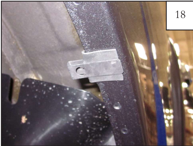
18 Install supplied long clips (CL1-0009) over the foam tabs.
