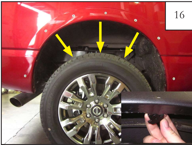
16 After removing the Factory flare, remove 3 factory installed clips.
