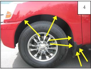
Remove factory mud flaps if installed, and one extra unpainted screw above mud flap. Also remove screw located at front of fender just above bumper. If no mud flaps were removed, remove two unpainted factory screws per side. Save for reinstallation.
