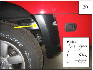
Slide a Clip (CL1-0005) over the door lip at the top of the door where the indent in the flare is. (The clip will be at a slight angle). Start Screw (SW1-0050). *Do not fully tighten screws.*
