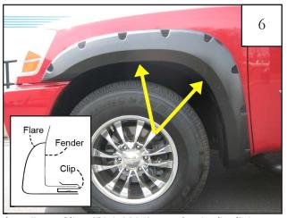
Install two Clips (CL1-0005) over fender lip, lining up the hole in clips with the holes in flare. Start Screws (SW1-0050) in each Clip. *Do not fully tighten screws*.
