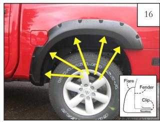
**Driver Side Flare:** Install five Clips (CL1-0005) over fender lip, lining up the hole in clips with the holes in flare. Start Screws (SW1-0050) in each Clip. *Do not fully tighten screws.*
