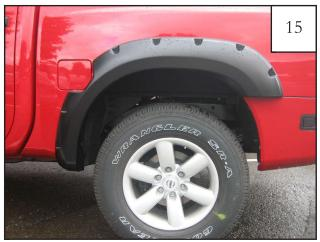
**Driver Side Flare:** Hold (LR) flare in position on fender with moderate pressure. Ensure the notch in the flare is positioned correctly with the gas door.
