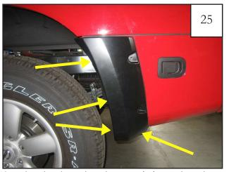
Insuring the door piece is properly located on door, apply moderate pressure to outside surface of flare, and tighten all screws, starting with the lowermost screw and moving up the part.
