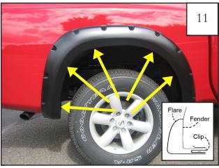
Passenger Side Flare: Install five Clips (CL1-0005) over fender lip, lining up the hole in Clips with the holes in flare. Start Screws (SW1-0050) in each Clip. Do not fully tighten screws.
