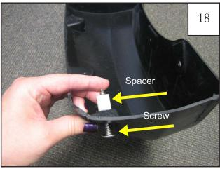
On the bottom of the door, pry out the Christmas Tree fastener. Open access door. Remove edge protector from door lip and discard. Insert two plastic grommets into the square holes on the edge of the door and one into the Christmas tree hole. Insert the supplied Screw (SW1-0034) through bottom hole in flare, and slide the supplied Spacer (SP1-0004) onto Screw on inside of flare
