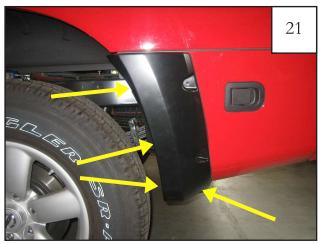
Insuring the door piece is properly located on door, apply moderate pressure to outside surface of flare, and tighten all screws, starting with the lowermost screw and moving up the part.
