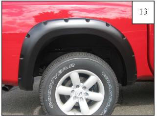
Passenger Side Flare: Completed rear flare installation.
