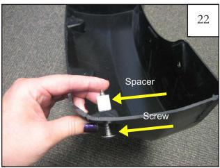
Remove factory mudflap and save the hardware (Step 14). Pry out the factory grommet on the lower surface of the door and install a supplied grommet. Open access door. Remove edge protector from door lip and discard. Insert the supplied Screw (SW1-0034) through bottom hole in flare, and slide the supplied Spacer (SP1-0004) onto Screw on inside of flare
