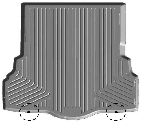
YOUR TRUNK LINER IS DESIGNED TO ALLOW ACCESS TO THE FACTORY CARGO NET ATTACHMENT POINTS LOCATED ALONG THE BACK WALL OF THE TRUNK AREA. TO ACCESS THESE LOCATIONS, YOU WILL NEED TO TRIM AWAY THE TWO LOWERED AREAS ON YOUR LINER THAT COVER THE ATTACHMENT POINTS (SHOWN CIRCLED ABOVE). TO TRIM, SIMPLY USE A PAIR OF HEAVY SHEARS OF A UTILITY KNIFE AND REMOVE THE LOWERED AREAS FROM THE LINER. YOUR TRUNK LINER WILL NOT FIT HYBRID FUSION MODELS.
