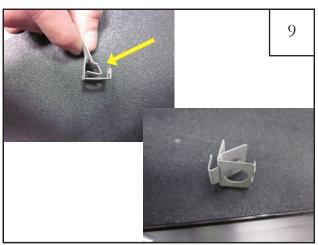
Assemble clip by connecting two provided parts CL1-0008 and CL1-0010 as shown. NOTE: *Do not fully snap clip together*
