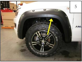
Place flare on vehicle and install one factory screw where shown to hold in place.
