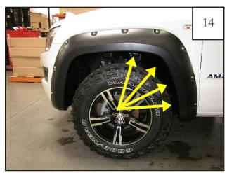
Using T-25 Torx bit, reinstall factory screws in 4 remaining Flare holes. Fully tighten all screws starting with the newly installed Screws (SW1-0058) in two forward hole locations while pressing in on flare to ensure it is snug against sheet metal.
