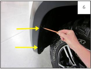
Using a grease pencil, mark the bumper cover through the 2 forward holes in flare.
