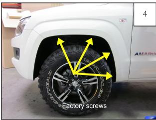
Using a T-45 Torx bit, remove four factory screws from the fender lip. Save screws for reinstallation. Remove flare by pulling part away from side of vehicle.
