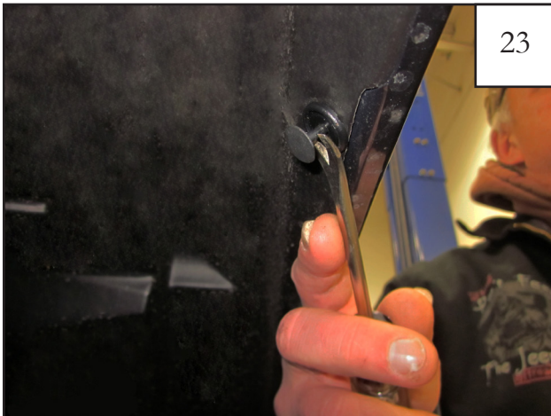
23 Using a pry tool, remove two plastic factory fasteners. Reference Step 22 for locations.
