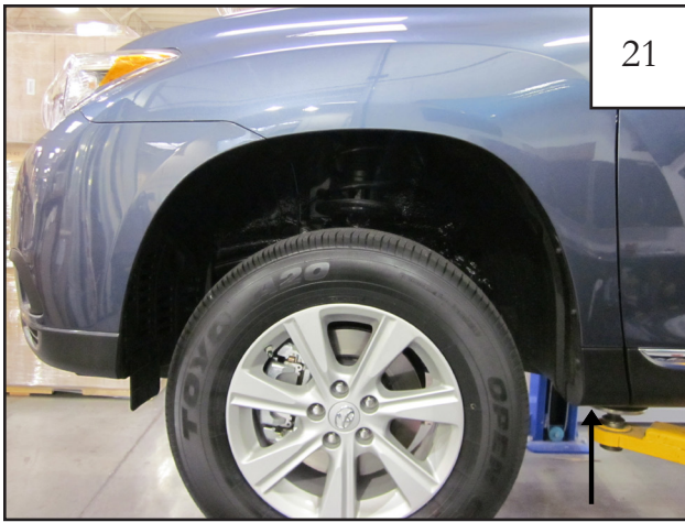
21 Using a pry tool, remove plastic factory fastener at lower rear of wheel well.
