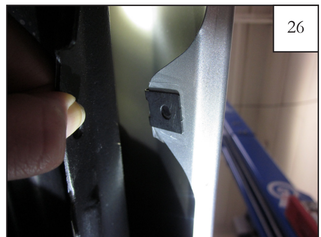
26 Slide Clip (CL1-0022) over factory hole locations behind wheel well liner over tab installed in previous step. Two locations. Reference Step 22 for locations.
