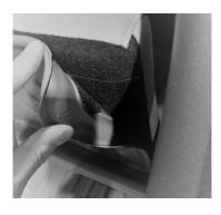
7. If your vehicle is equipped with a factory subwoofer, There is a trim groove molded in the liner to guide trimming.
