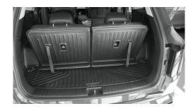
6. The liner at this point is fully installed and is ready to use. If the liner needs to be removed, grab the rectangular Velcro patches and hold them firmly in place as you pull the liner from the seat. This Velcro piece is intended to stay attached to the seat back and cargo floor to reduce ware from the liner being installed and reinstalled for cleaning.
