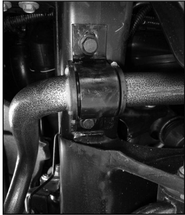
1. Remove the skid plate to gain access to the factory sway bar. Keep all the hardware to reinstall the skid plate.
