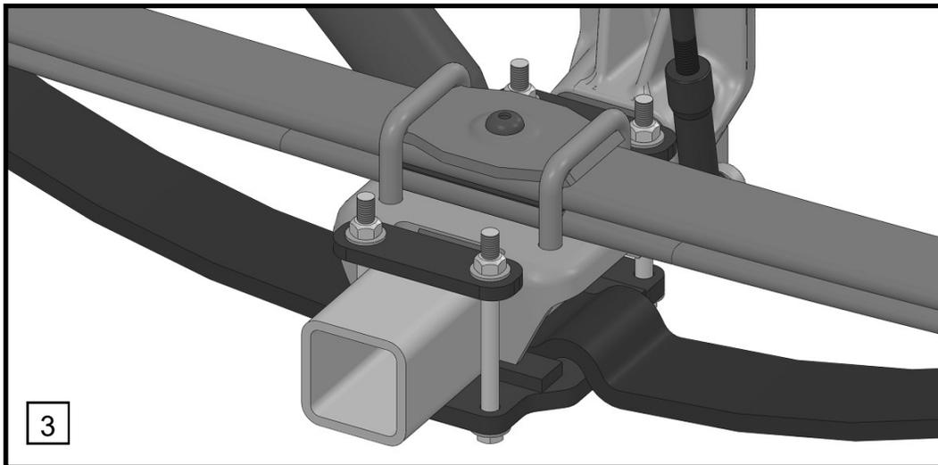
3. Place the Hellwig spring on top of the base plate with the hump centered on the plate as shown in photo 3.
