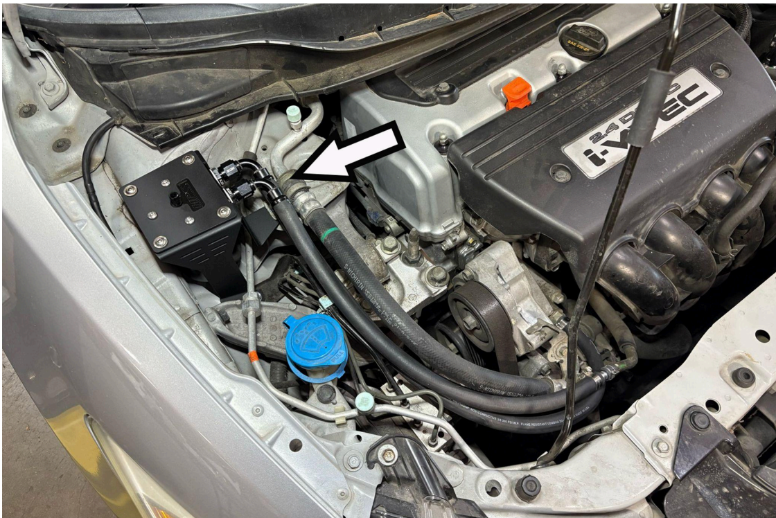
14. Fasten the 90 degree AN fitting to the left side adapter of the oil catch can.
