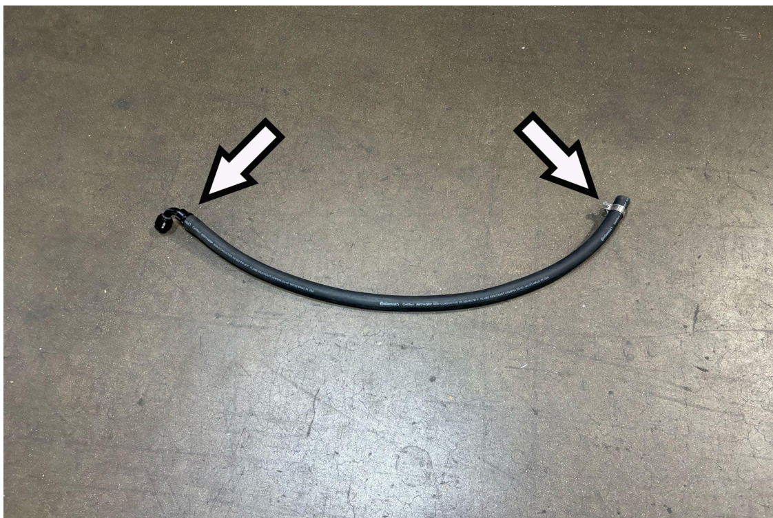
10. Secure one 90 degree AN fitting to the 25-inch push-on hose. Then, attach an FIC clamp to the other end of the hose.
