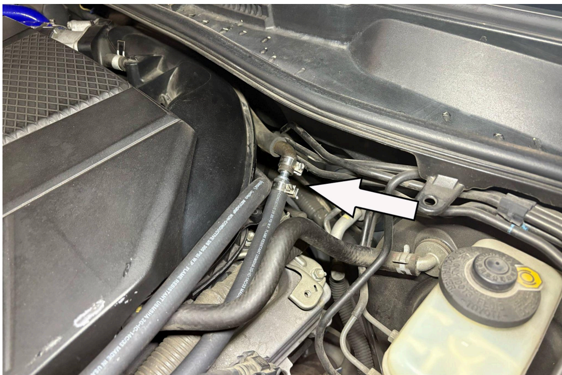
14. Connect the factory PCV hose to the barbed AN hose and secure it using the remaining fuel injection clamp.
