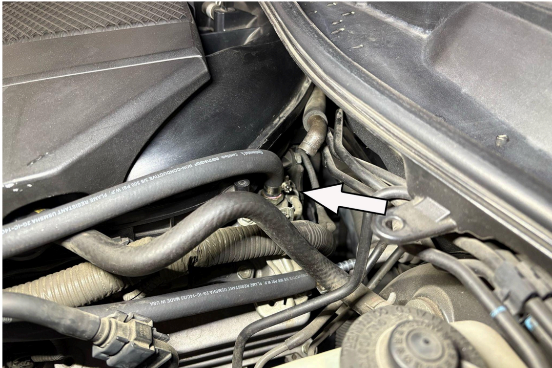
13. Secure the AN hose without the barb fitting onto the PCV valve using the fuel injection clamp.
