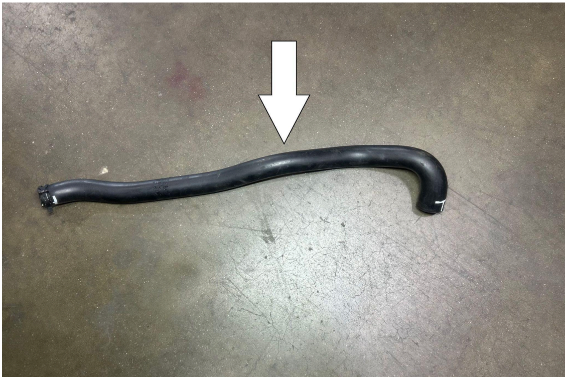
6. Remove the crankcase vent hose from the vehicle.
