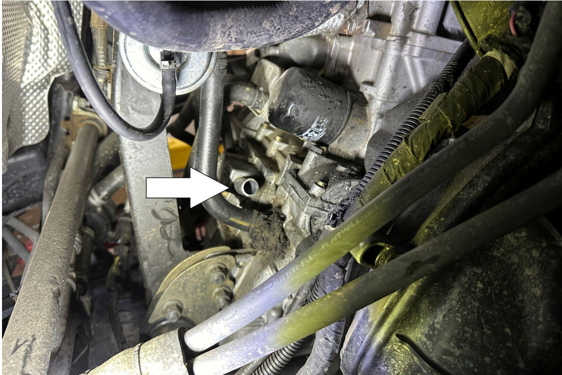
5. Disconnect the opposite side of the crankcase vent hose from the engine.
