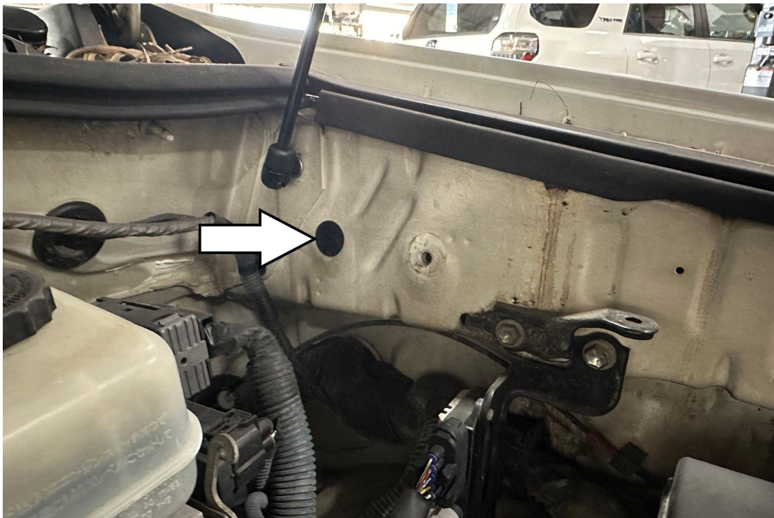
4. Remove the sticker from the inner fender.
