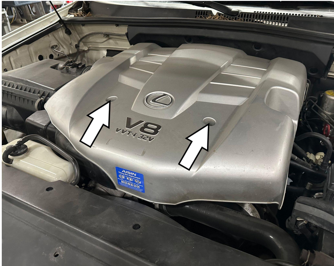
14. Reinstall the engine cover.
