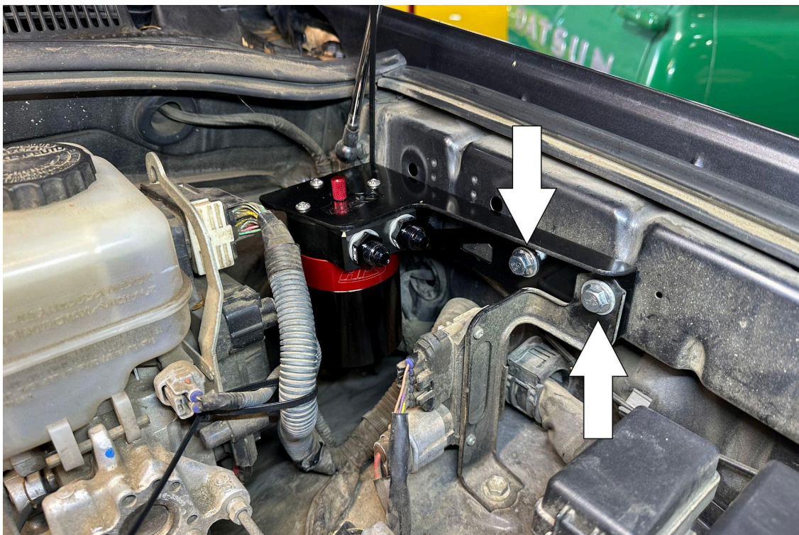
8. Install oil catch can with bracket to the drivers inner fender using two of each provided M8 bolts and washers.
