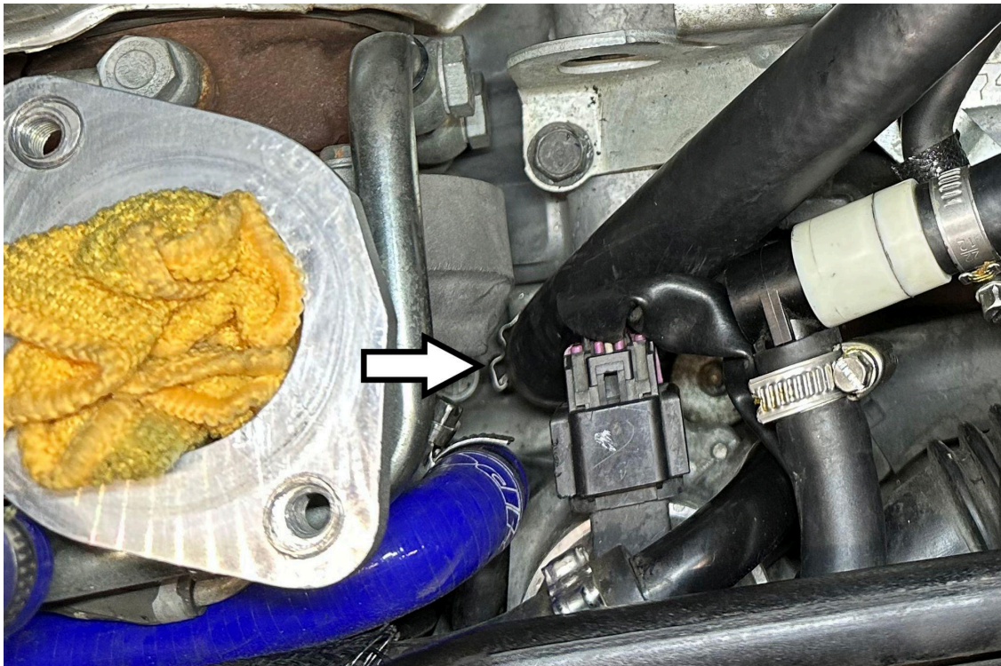
16. The original clamp installed on the PCV valve, when closed, will look like the picture above. Reconnect the black electrical connector.
