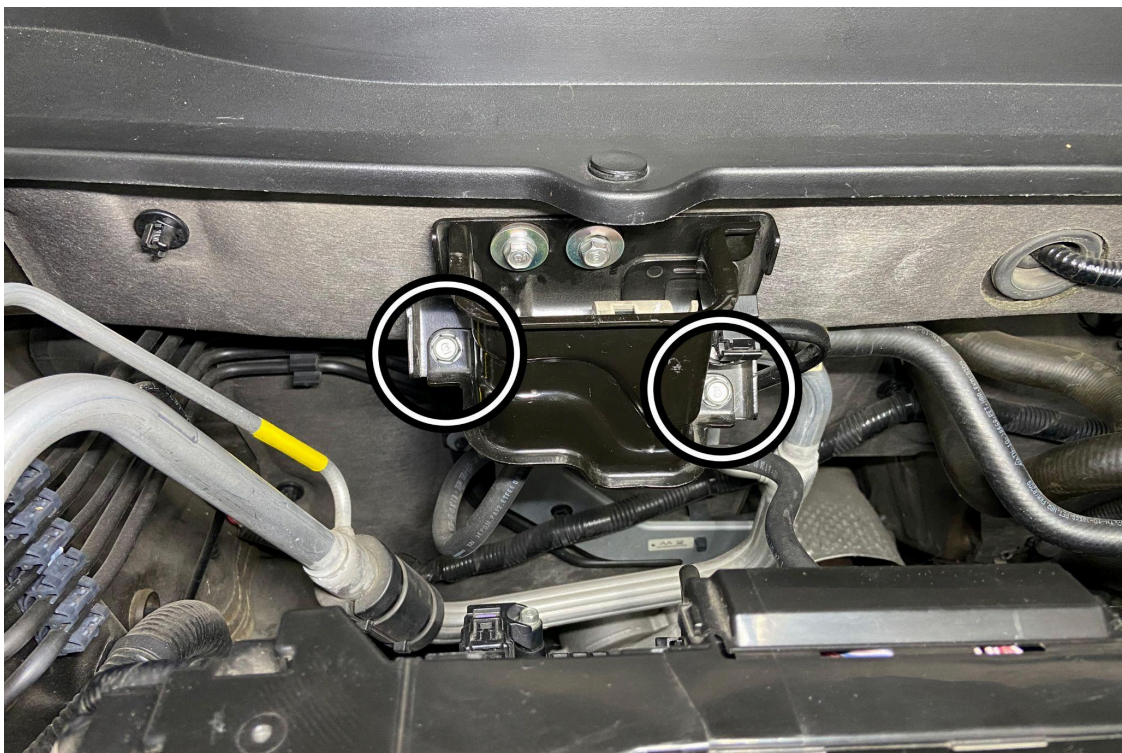
4. Remove the two 10mm bolts securing the fuel hose cover and remove it from the vehicle.
