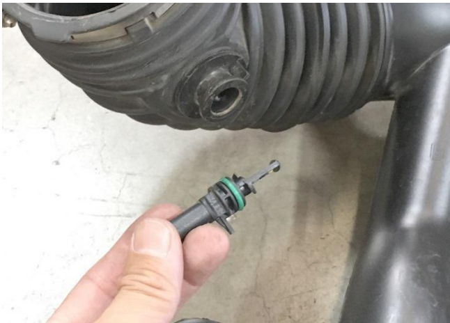
8. Remove the intake air temperature sensor by turning the sensor a 1/4th turn counter-clockwise.
