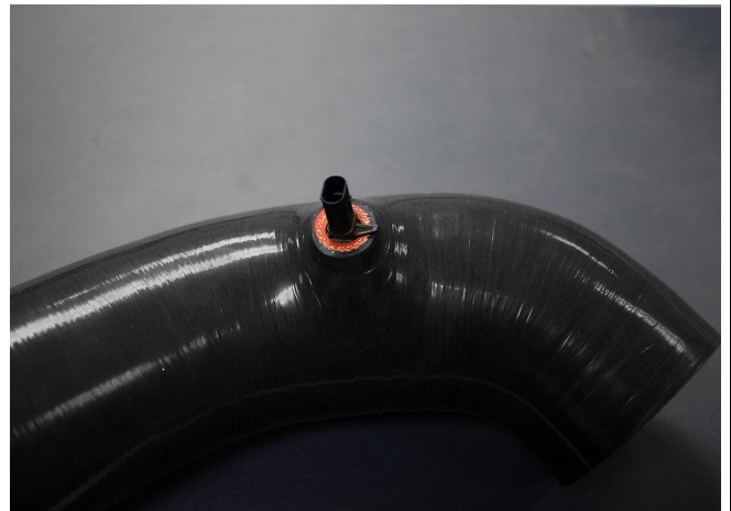
9. Install the intake air temperature sensor onto the HPS intake tube.
