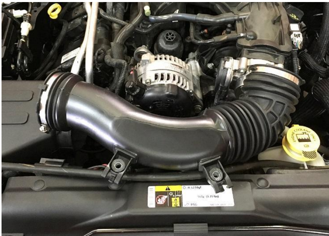
6. Disconnect both ends of the intake tube. Carefully lift up but do not remove it from the engine bay yet.
