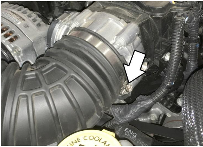
4. Loosen the hose clamp from the throttle body.
