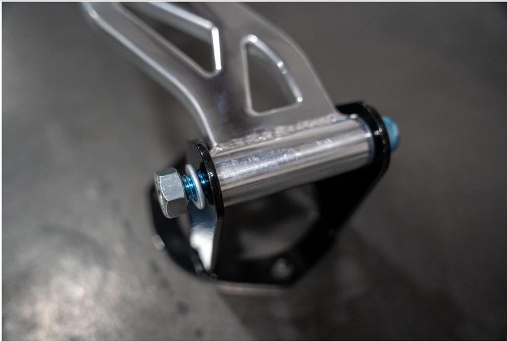
9. Torque down the M12 Allen bolts and the M12 nuts to 80 ft-lbs.
