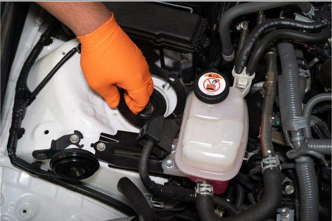
4. Remove the OEM strut tower plate on each side.
