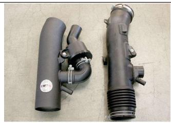
11. Remove and switch the stock sound generator onto to the HPS intake pipe. Reuse the factory bolt to secure the sound generator or use the provided M6 bolt and nut to secure the generator if your HPS intake pipe does not have a threaded mount bracket.
