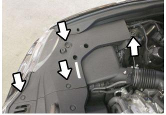
3. Release the four rivets by pushing the center of the rivets then remove the plastic panel covering the air box.
