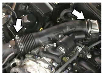
5. Loosen the hose clamps on the throttle body and air box.
