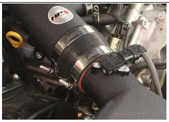
13. Connect the opposite end of the intake pipe to the air box.
