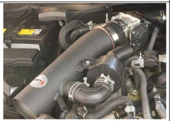
12. Insert the intake into the coupler on the throttle body.
