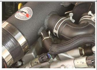
14. Reinstall the stock breather hose into the intake.
