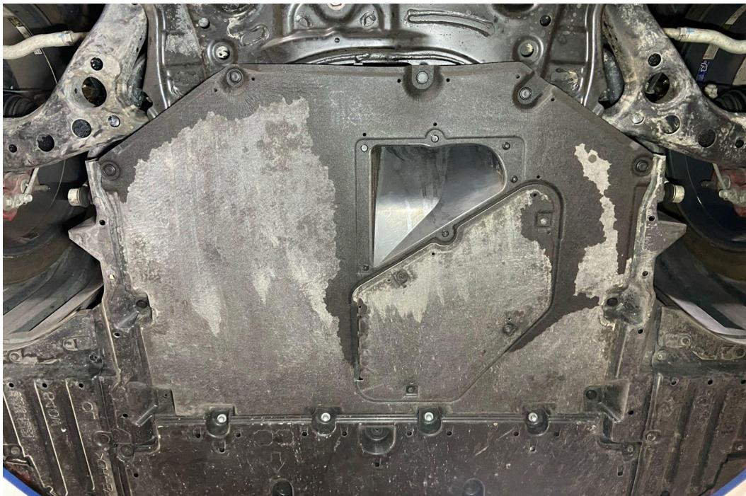
10. Reinstall the under tray back onto the vehicle.
