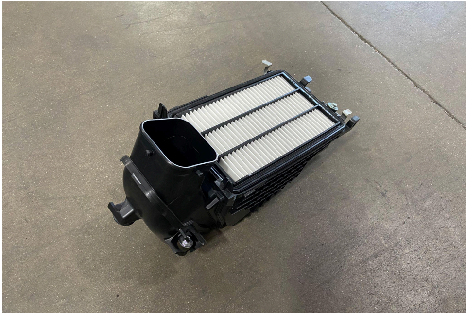
10. Lift the lower air box and remove it from the vehicle.
