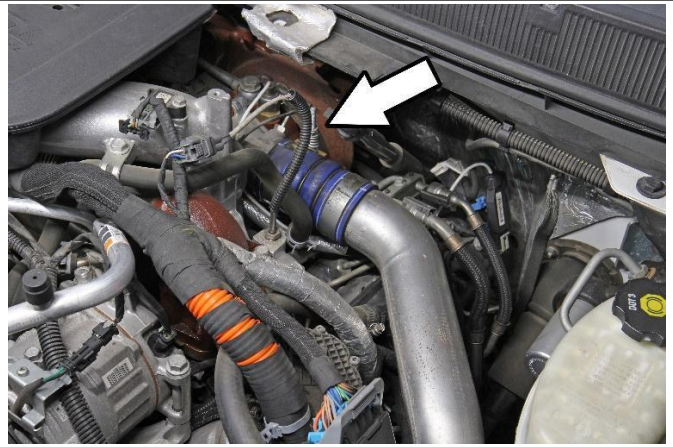
19. Loosen the hose clamp securing the hot side charge pipe from the turbo outlet.
