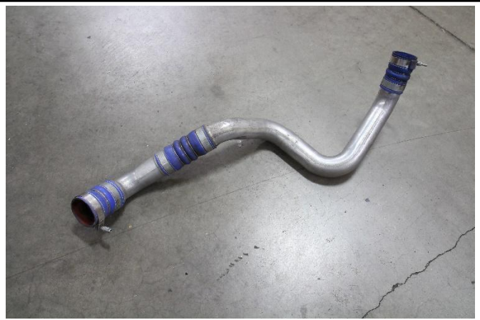
21. With an assistant, remove the hot side charge pipe by guiding the pipe towards the top.
