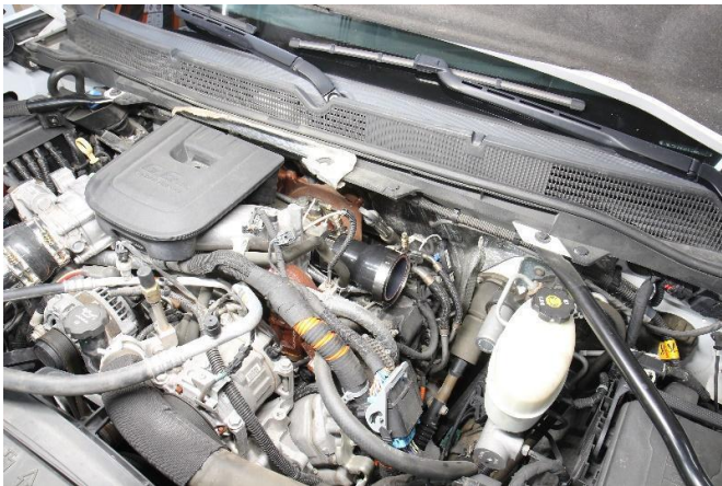
22. Install the long reducer coupler, along with the provided T-bolt clamps onto the turbo outlet.
