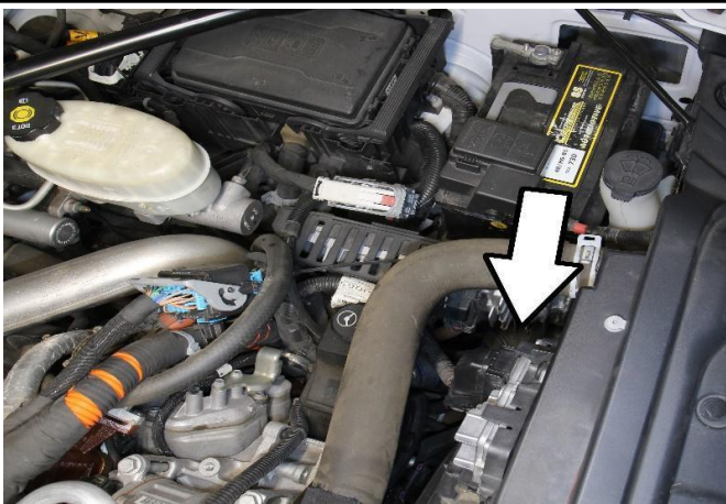
20. In this case, the hose clamp was facing the top of the engine. Loosen the hose clamp securing the charge pipe to the intercooler from the top of the engine using a long extension.
