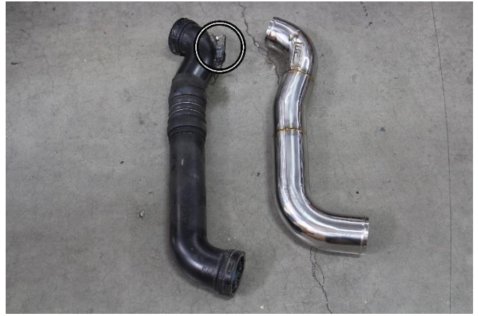
13. Remove the temperature sensor from the factory charge pipe and install it onto the HPS charge pipe.
