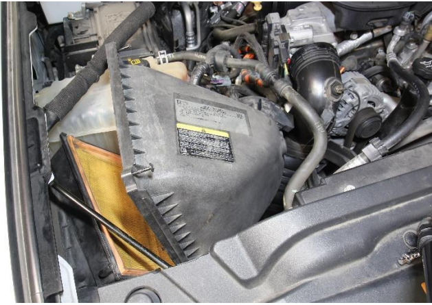
6. Remove the upper air box assembly from the vehicle.
