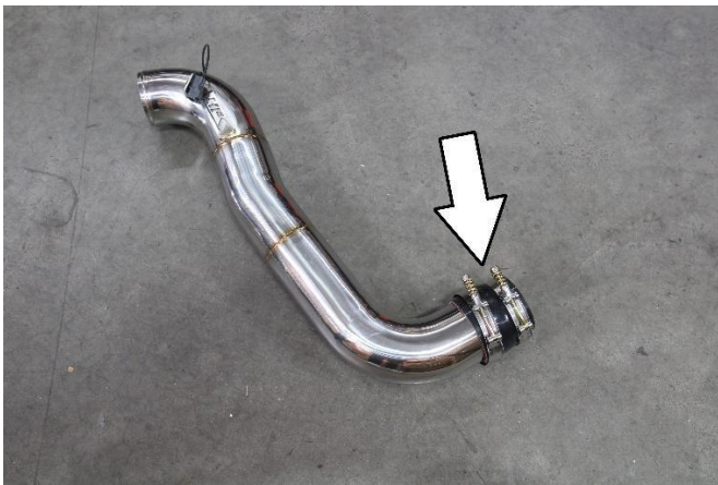
14. Insert the provided silicone reducer coupler, along with the T-bolt clamps, onto the end of the charge pipe as shown above.
