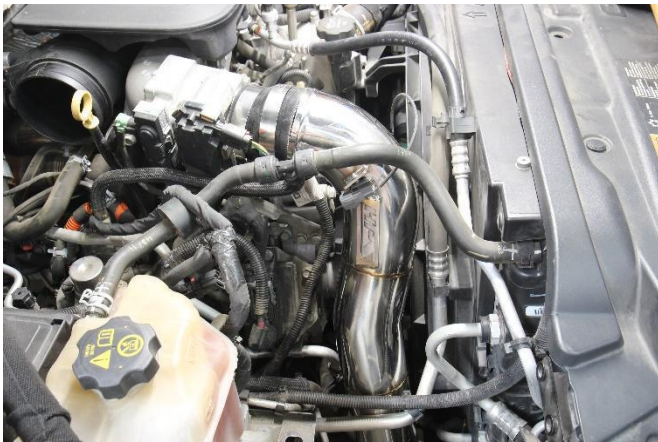
16. Insert the HPS charge pipe into the vehicle by inserting the charge pipe onto the intercooler side first.
