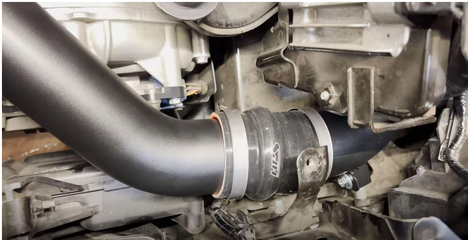
37. Insert and secure the upper HPS charge pipe assembly to the HPS extension.
