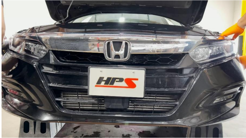
38. Reinstall the front bumper back onto the vehicle as well as the air box assembly.
