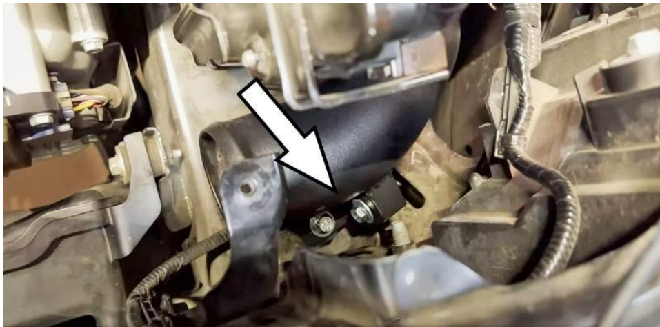
36. Insert and secure the provided "L" bracket onto the charge pipe using the two M6x12mm bolts and washers.
