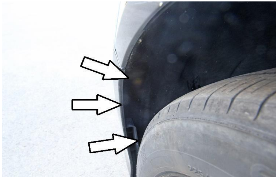
29. Remove the plastic retaining clip and the two screws securing the inner wheel liner from the bumper. Move the inner liner aside and remove the one screw securing the bumper to the fender.
