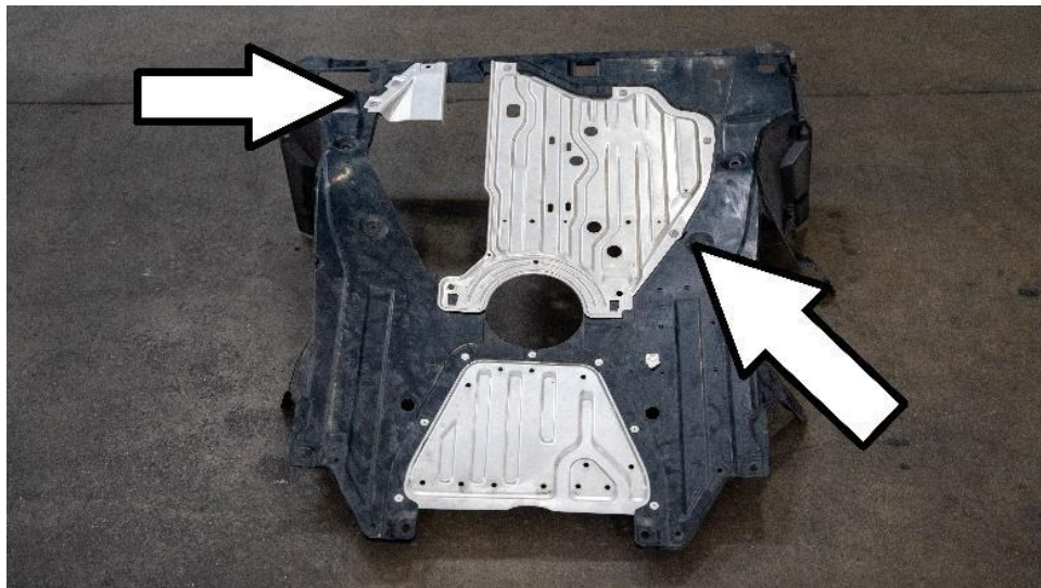
39. Loosen the 9 screws to remove the two pieces of aluminum undertray located under the vehicle.
