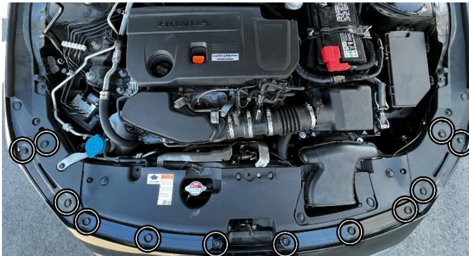
27. Remove the 12 retaining clips securing the upper part of the bumper shown in the image above.
