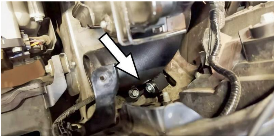
20. Insert and secure the provided "L" bracket onto the charge pipe using the two M6x12mm bolts and washers.
