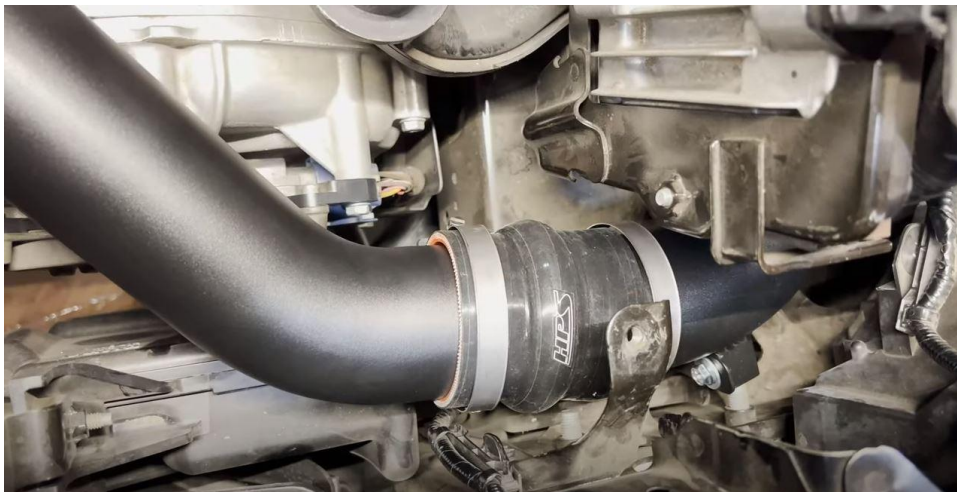
21. Insert and secure the upper HPS charge pipe assembly to the HPS extension.
