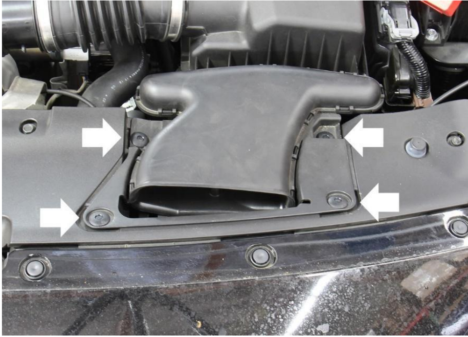
10. Push down the center of the 4 button clips to remove the air duct from the engine bay.
