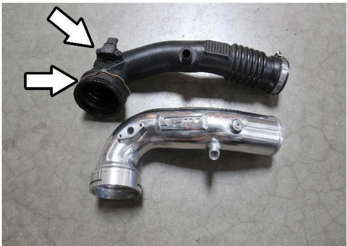
6. Remove the factory retaining clip and air temperature sensor from the factory charge pipe.
