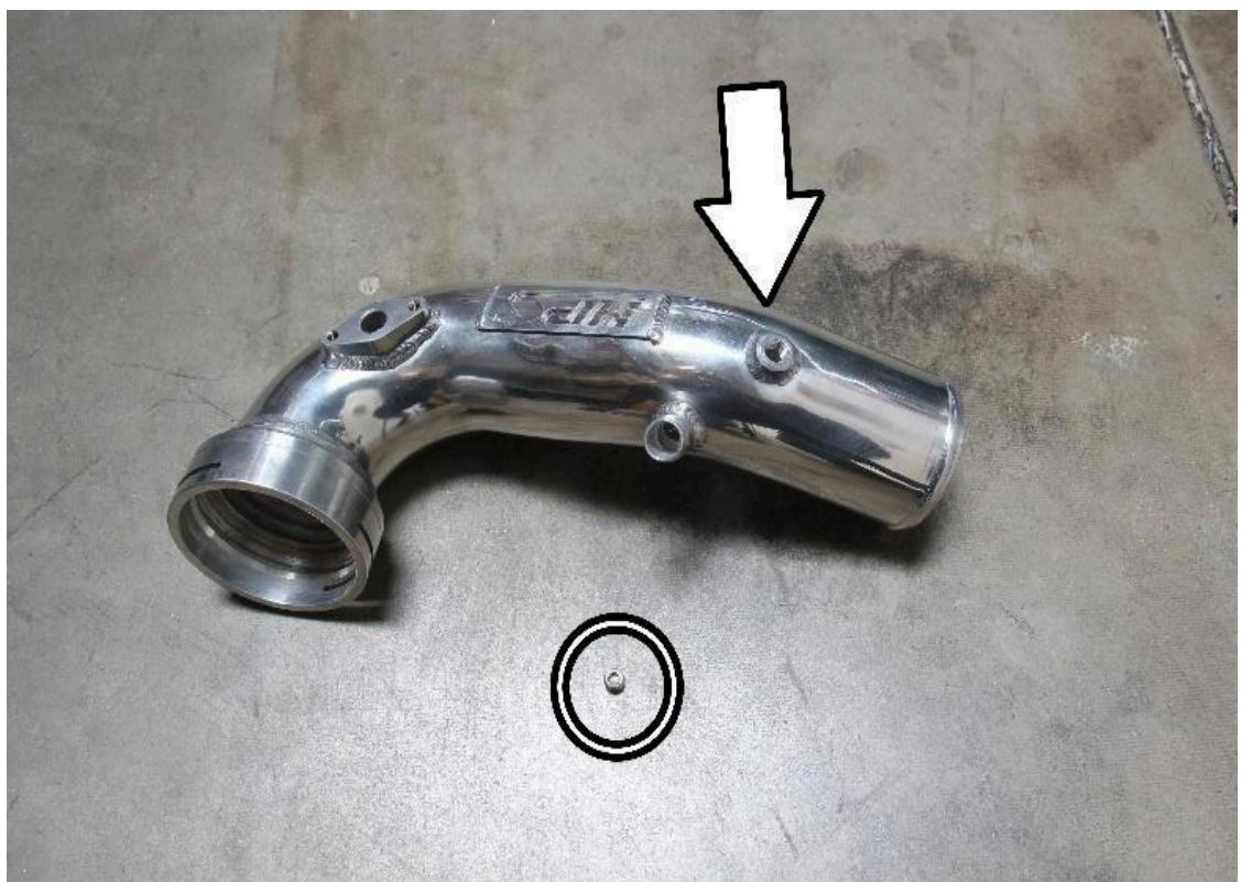
5. Secure the provided NPT plug into the HPS charge pipe.
