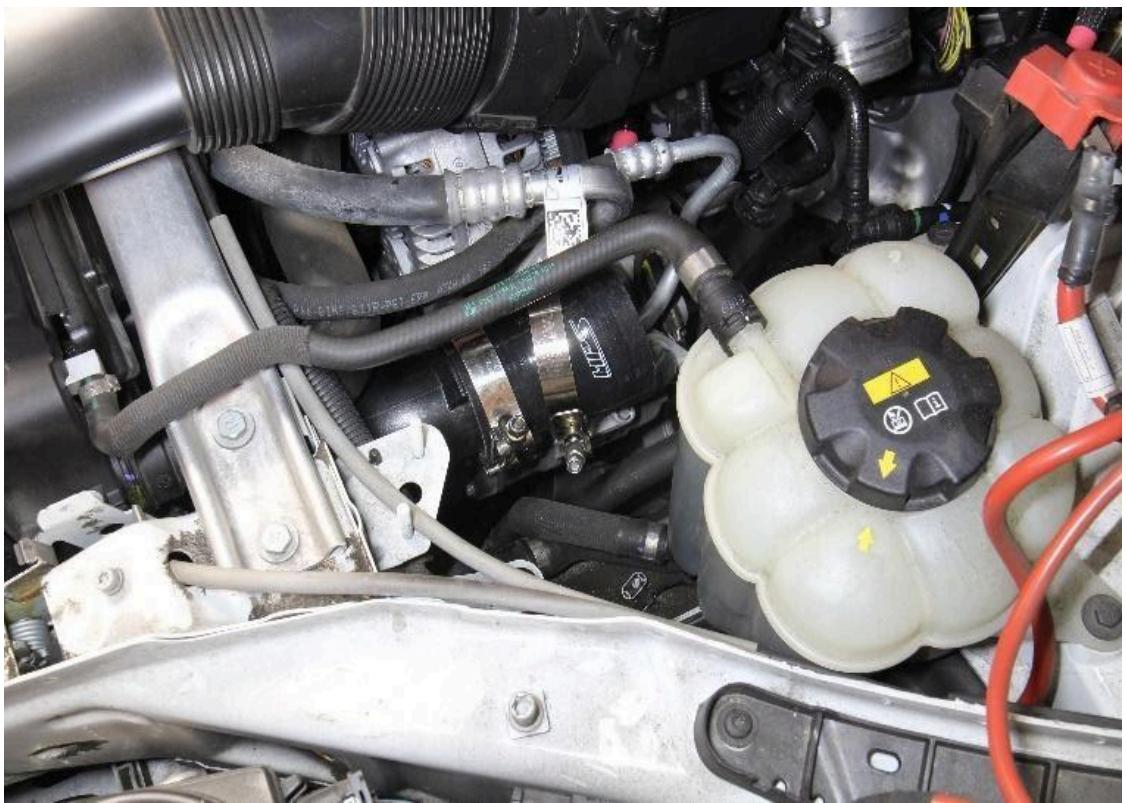
9. Install the coupler onto the intercooler outlet using the provided T-bolt clamps.
