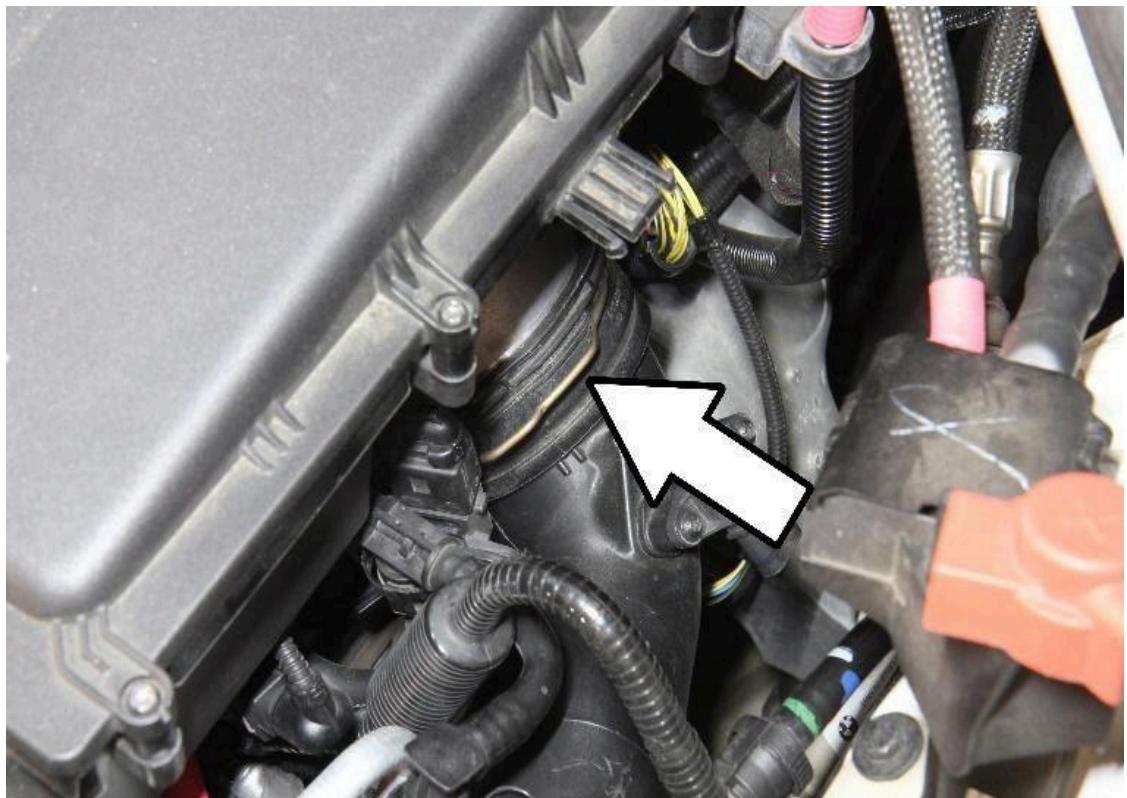
4. With a flathead screwdriver, lift the retaining clip securing the charge pipe to the throttle body and remove the factory charge pipe from the vehicle.
