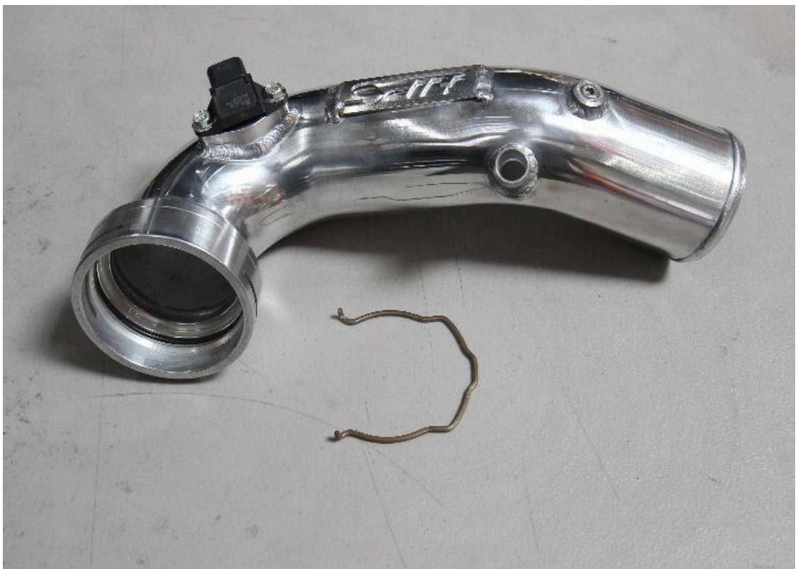
8. Secure the air temperature sensor onto the HPS charge pipe using the provided M6 bolts. Then place the O-ring into the quick connect.
