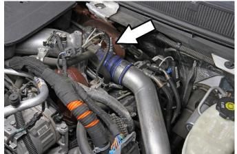
2. Loosen the hose clamp securing the hot side charge pipe from the turbo outlet.
