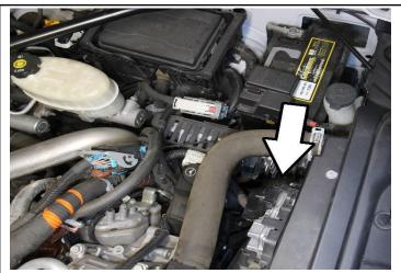
3. In this case, the hose clamp was facing the top of the engine. Loosen the hose clamp securing the charge pipe to the intercooler from the top of engine using a long extension.
