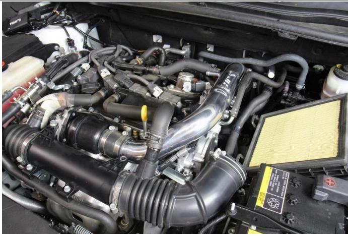
16. Insert and secure the charge pipe into the vehicle.
