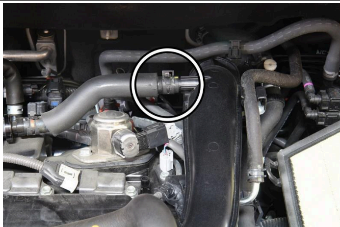
8. Depress the spring clamp securing the breather hose from the stock charge pipe and disconnect the hose from the charge pipe.
