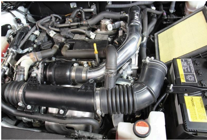
18. Re-insert the stock intake breather hose onto the intake breather barb.
