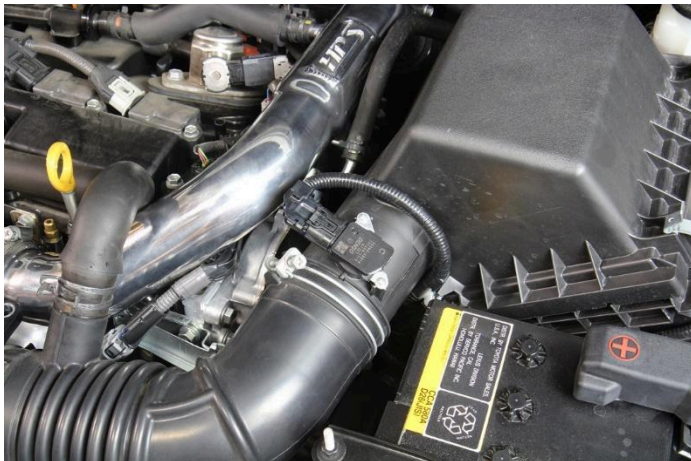
20. Insert the MAF sensor connector harness clip back onto the upper air box and re-connect the electrical harness onto the MAF sensor.
