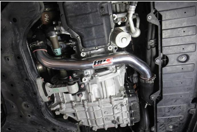
12. Insert the HPS intercooler pipe into the couplers and adjust the hoses to the proper position.
