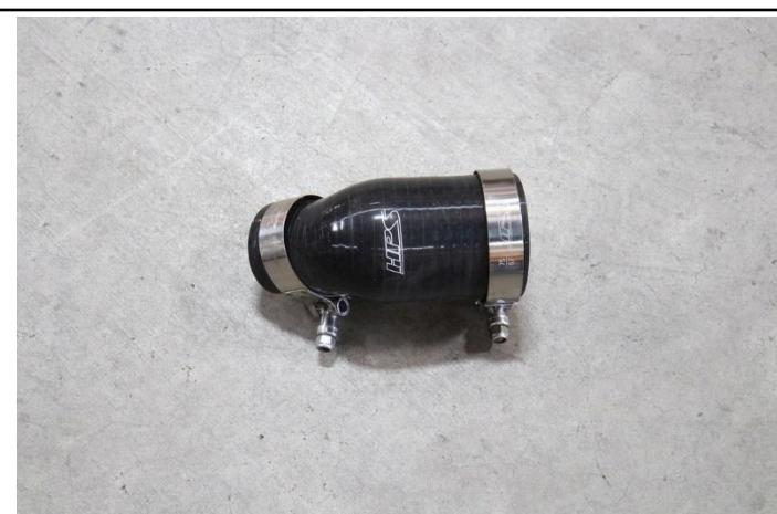
8. Attach the t-bolts clamps provided in the kit onto the small 45-degree reducer coupler.
