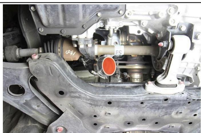
9. Insert the reducer coupler along with the provided t-bolt clamps onto the turbo inlet. Do not tighten the clamps yet because the hose will still need to be adjusted to the proper position.
