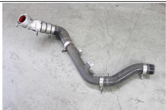
7. Remove the stock charge pipe assembly from the vehicle.
