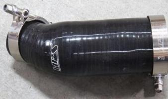
10. Attach the remaining t-bolt clamps onto the other 45-degree reducer coupler.
