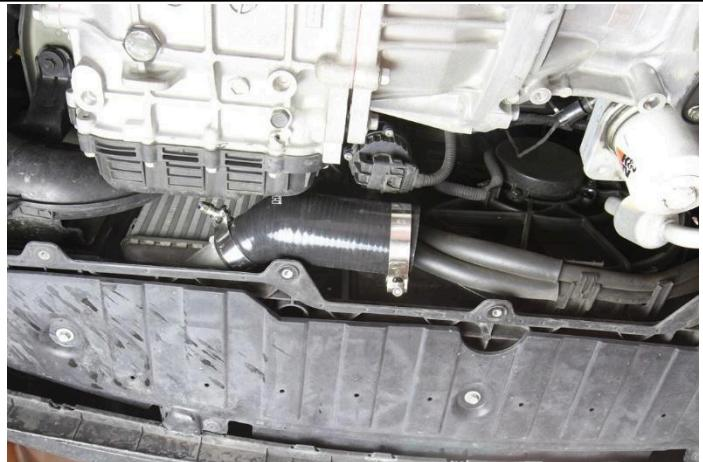
11. Insert the 45-degree reducer coupler along with the t-bolt clamps onto the intercooler. Do not tighten the clamps yet because the hose will still need to be adjusted to the proper position.
