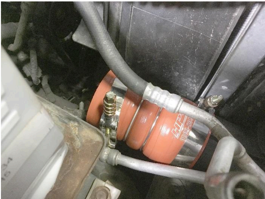
12. Install hose "ORCH-HOT-101" along with the provided spring loaded T-bolt clamps onto the passenger side charge inlet.
