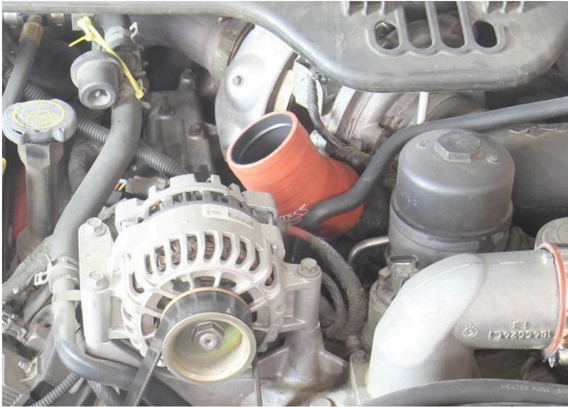
11. Insert hose "ORCH-HOT-102" onto the turbocharge outlet. Loosely place the small spring loaded T-bolt clamps onto the hose.
