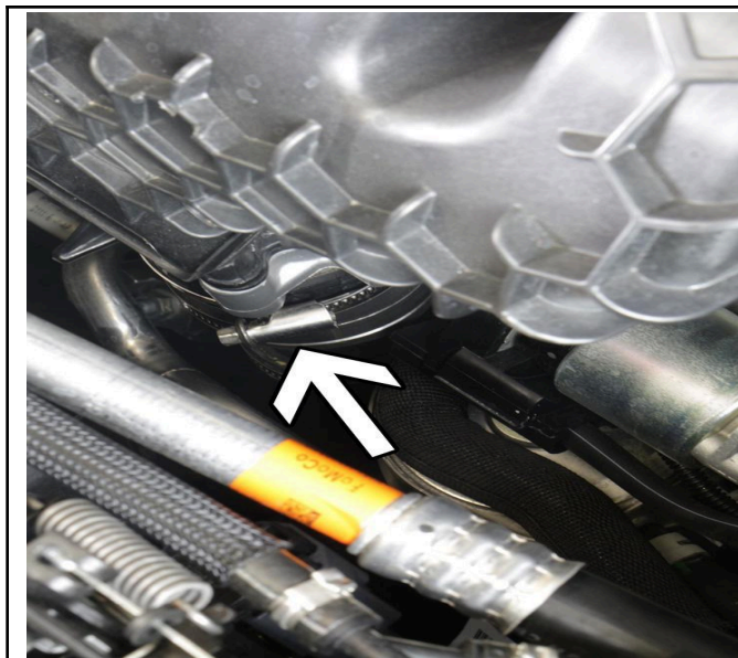
2. Loosen the hose clamp securing the throttle body.
