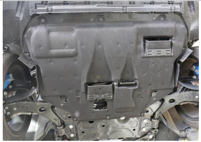
15. Re-install the undercover tray back onto the vehicle.
