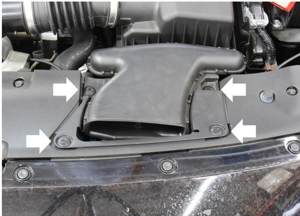
7. Push down the center of the 4 button clips to remove the air duct from the engine bay.
