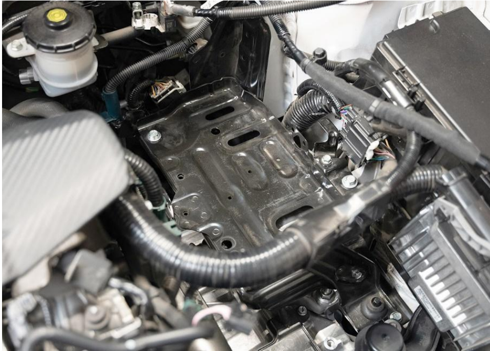
26. Reinstall the battery tray and battery.
