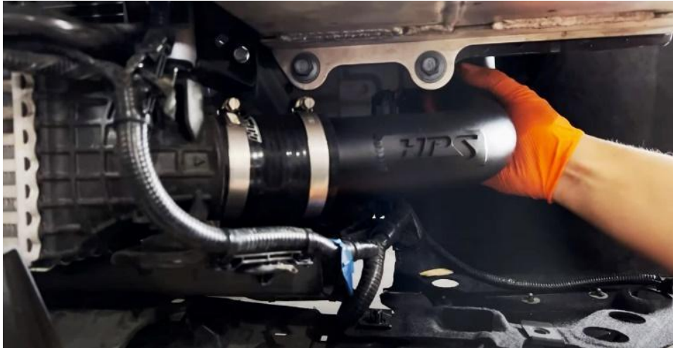
35. Insert the HPS cold side charge pipe into the vehicle.
