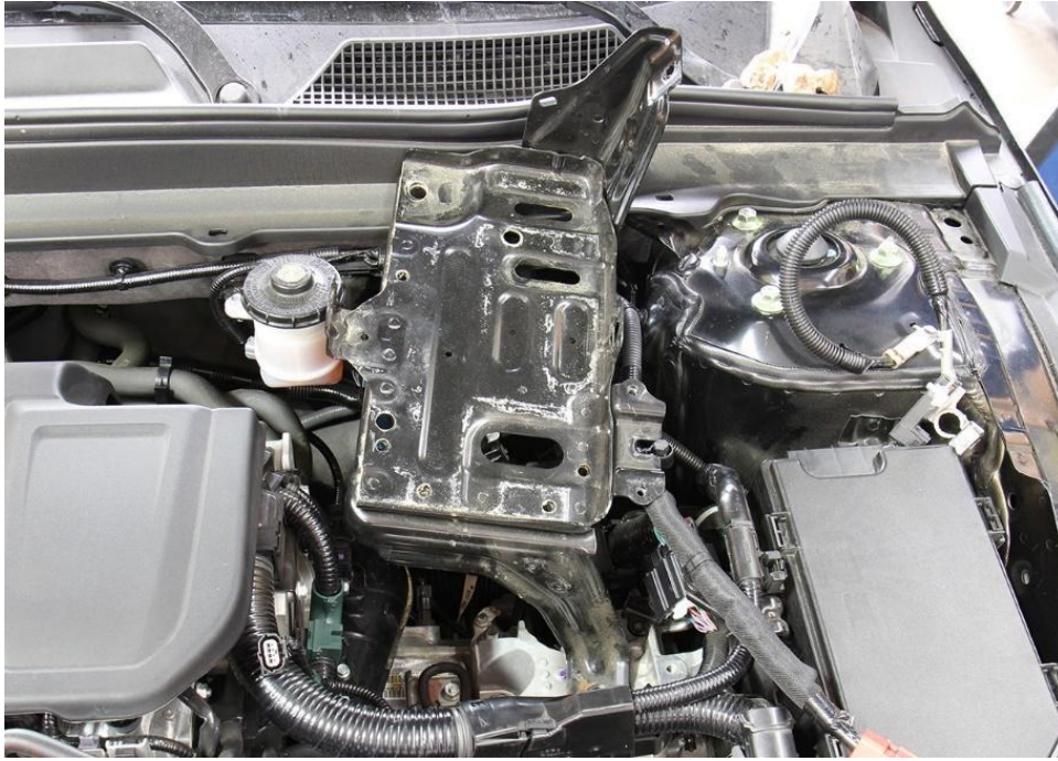
12. Carefully remove the battery tray from the engine bay.
