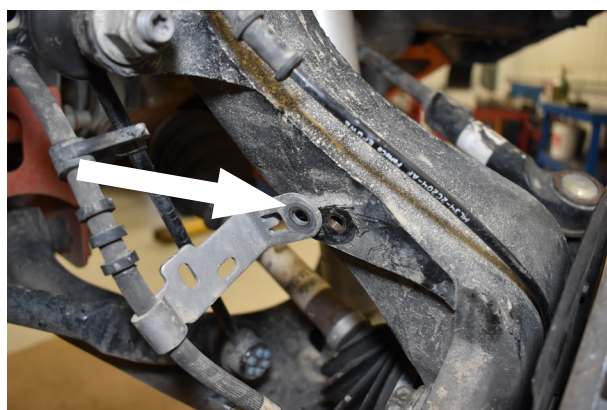
Fig. 3: Disconnect Brake line bracket.
