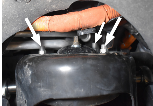
Fig.9: Remove the 3 Strut nuts.
