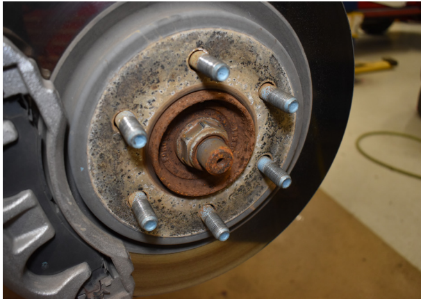
Fig.5: Remove Axle nut.
