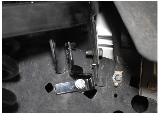
Fig. 24: Install sensor bracket to frame.
