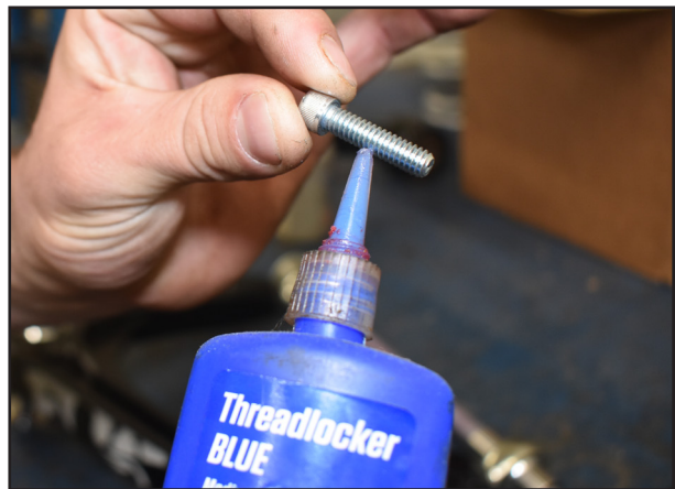
Fig. 17: Loctite pinch bolt threads.
