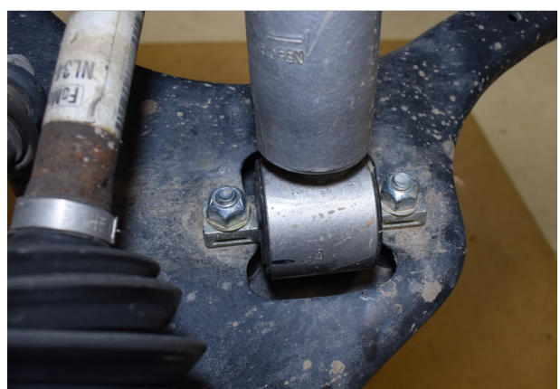
Fig.8: Disconnect sway bar link.
