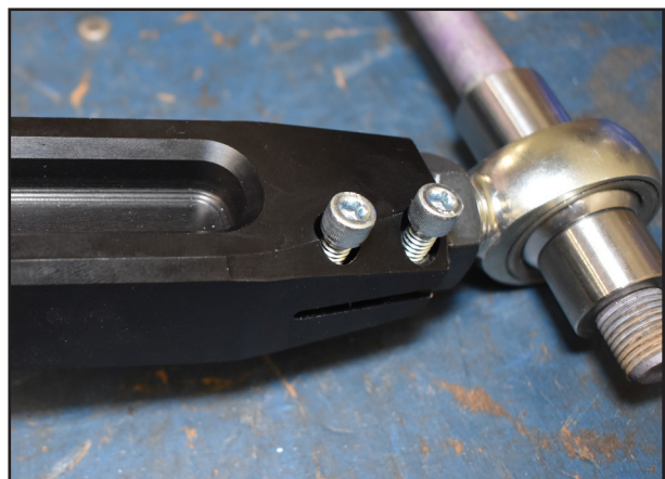
Fig. 18: Install pinch bolts.
