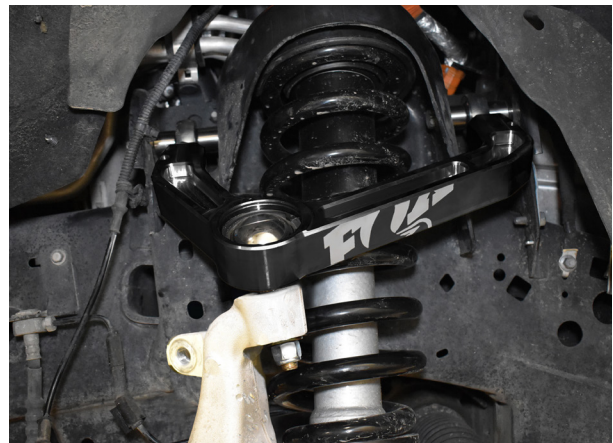
Fig. 21: Connect UCA to knuckle.
