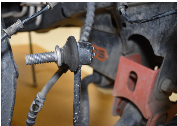
Fig.7: Disconnect sway bar link.
