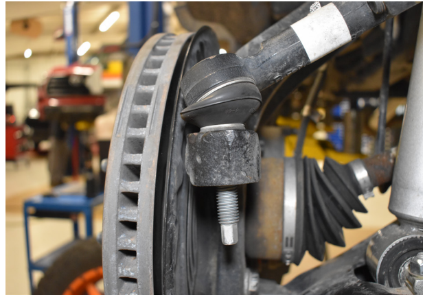
Fig.6: Disconnect the tie rod end.
